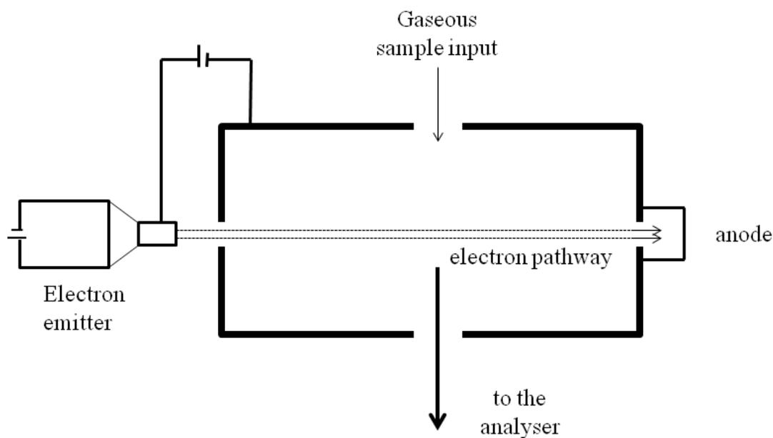
Figure 1.5: Electron ionisation source from a mass spectrometer.
