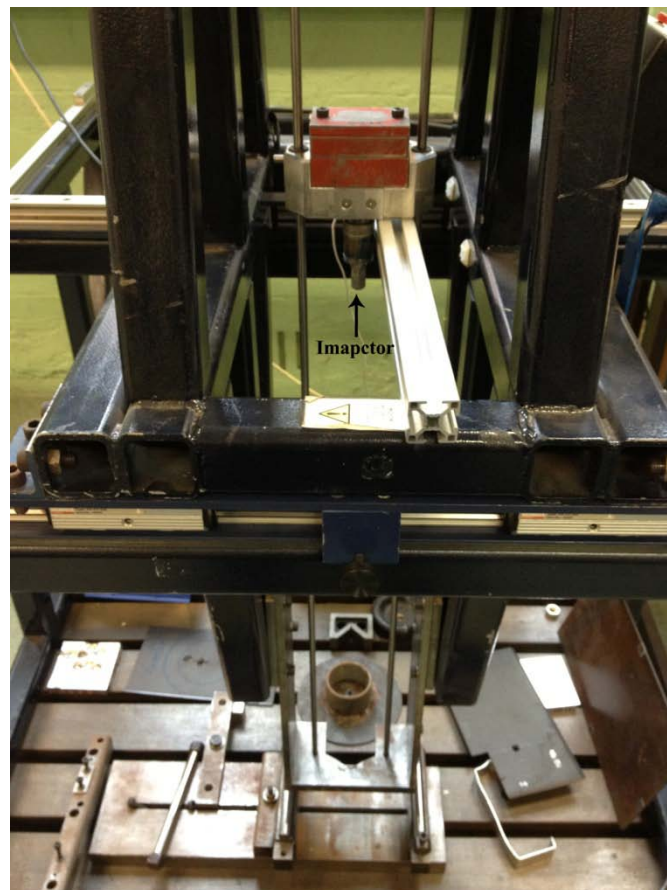
Figure 4.10: The impact test apparatus.
