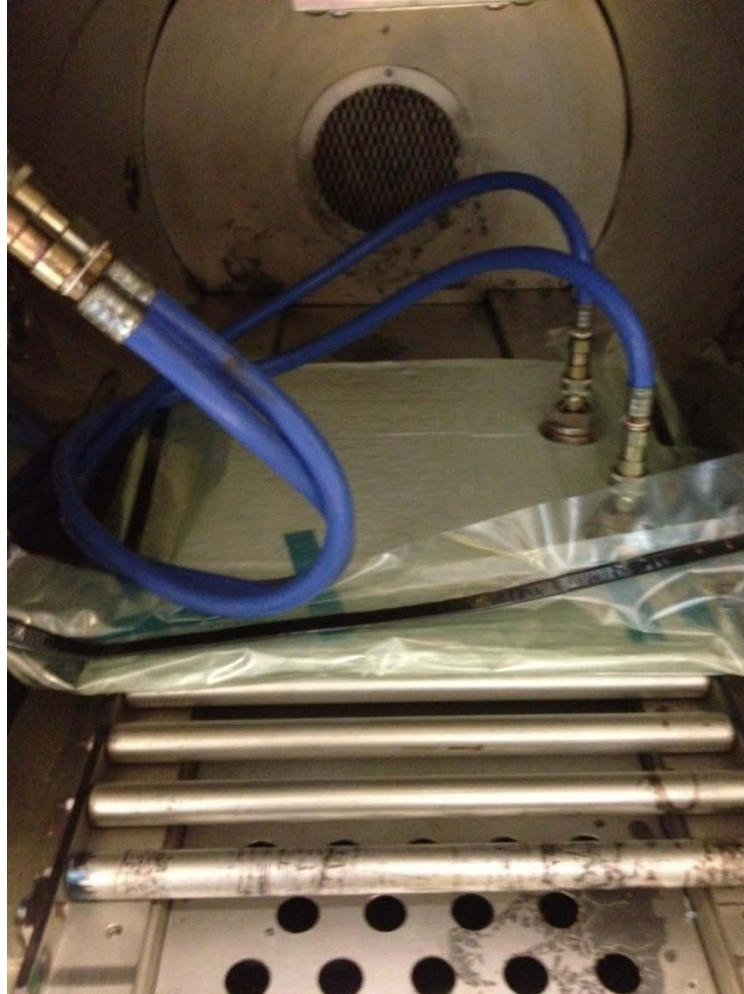
Figure 4.5: Curing process in autoclave.
