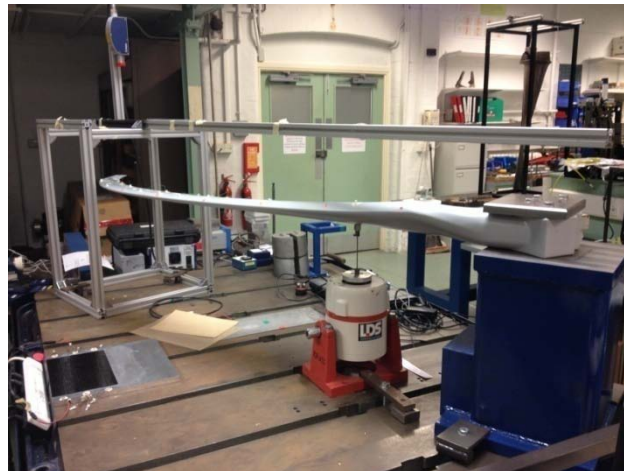
Figure 5.1: The geometric boundary condition of the wind turbine blade.
