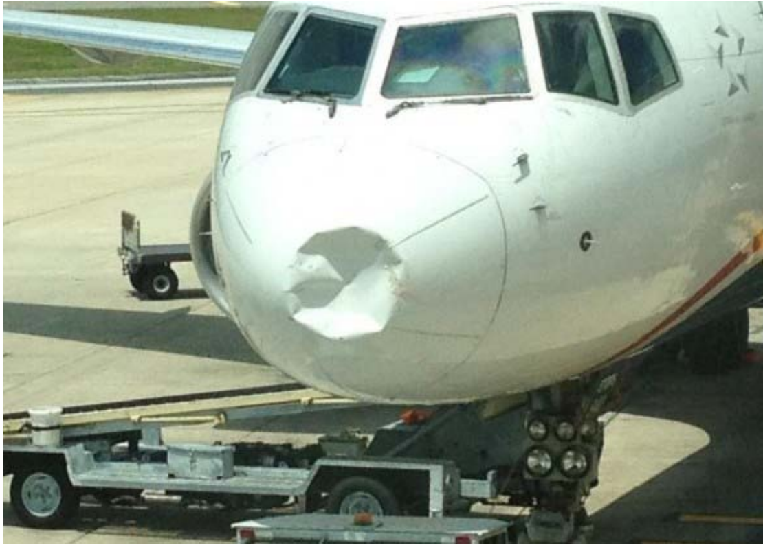
Figure 1.2: Bird strike on Boeing 757 with Radome Damage [12].
