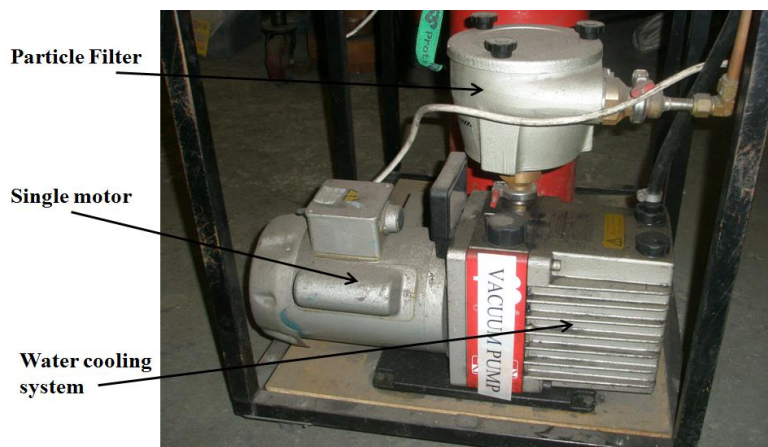
Figure 3.9 Edwards E1M18' Vacuum pump A for Test vessel 1
