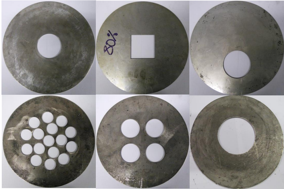
Figure 3.5 Sample of different configuration of the vent orifice Grid-Plates
