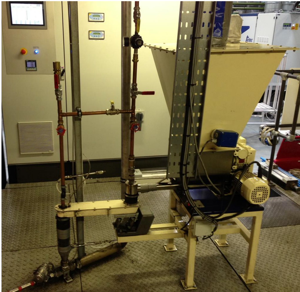
Figure 3.9. Fuel feeder, with feed storage hopper, screw feeder, vibrating tray, venturi feeder as well as the primary bypass line used to eliminate air ingress.
