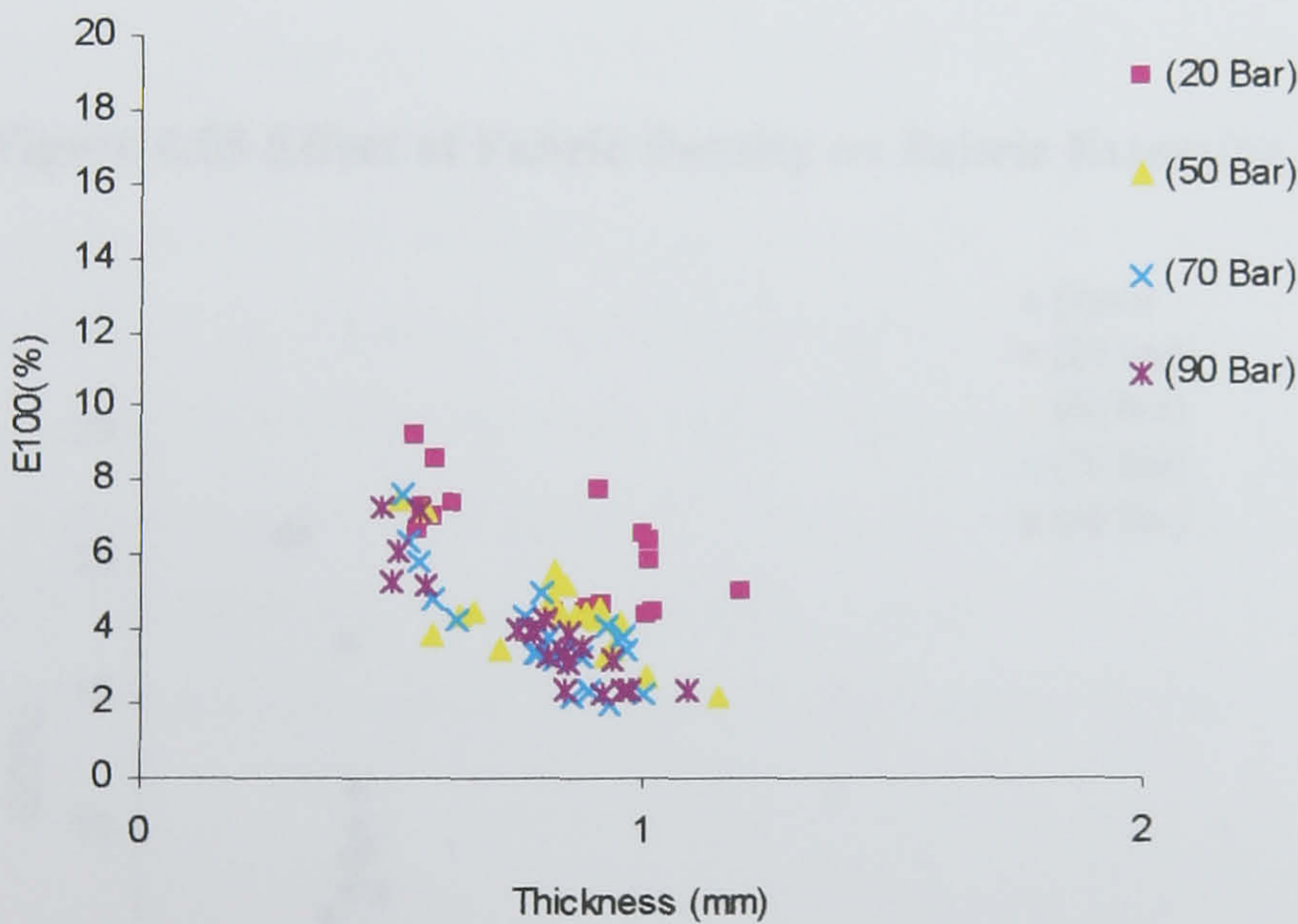
Figure 4.54 Effect of Thickness on Web and Fabric Extension at 100 gf/cm
