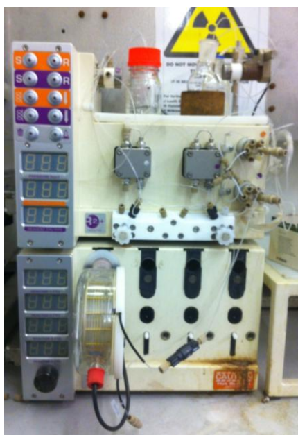
Figure 2. The Vapourtec R-Series system used for this project.
