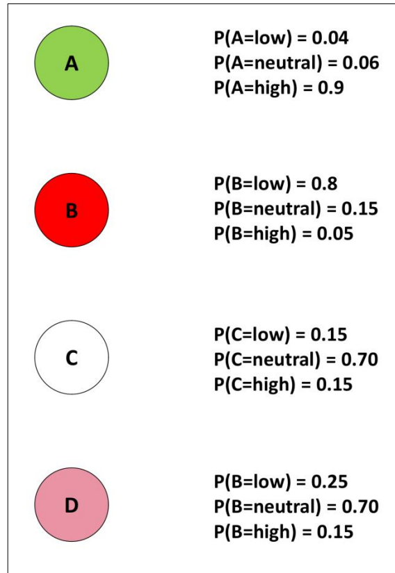
Figure 3-10: Schematic describing node colours and conditional probabilities. Node A has a high probability of being in the high concentration bin (0.9) therefore is coloured green. Node B has a high probability of being in a low concentration bin and is therefore coloured red. Node C has a high probability of being in a medium concentration bin and is therefore coloured white. In the case of equal probabilities across all concentration bins, the node would be coloured white. Node D has a slightly higher probability of being in a low concentration bin than a high concentration bin and is therefore coloured pink.
