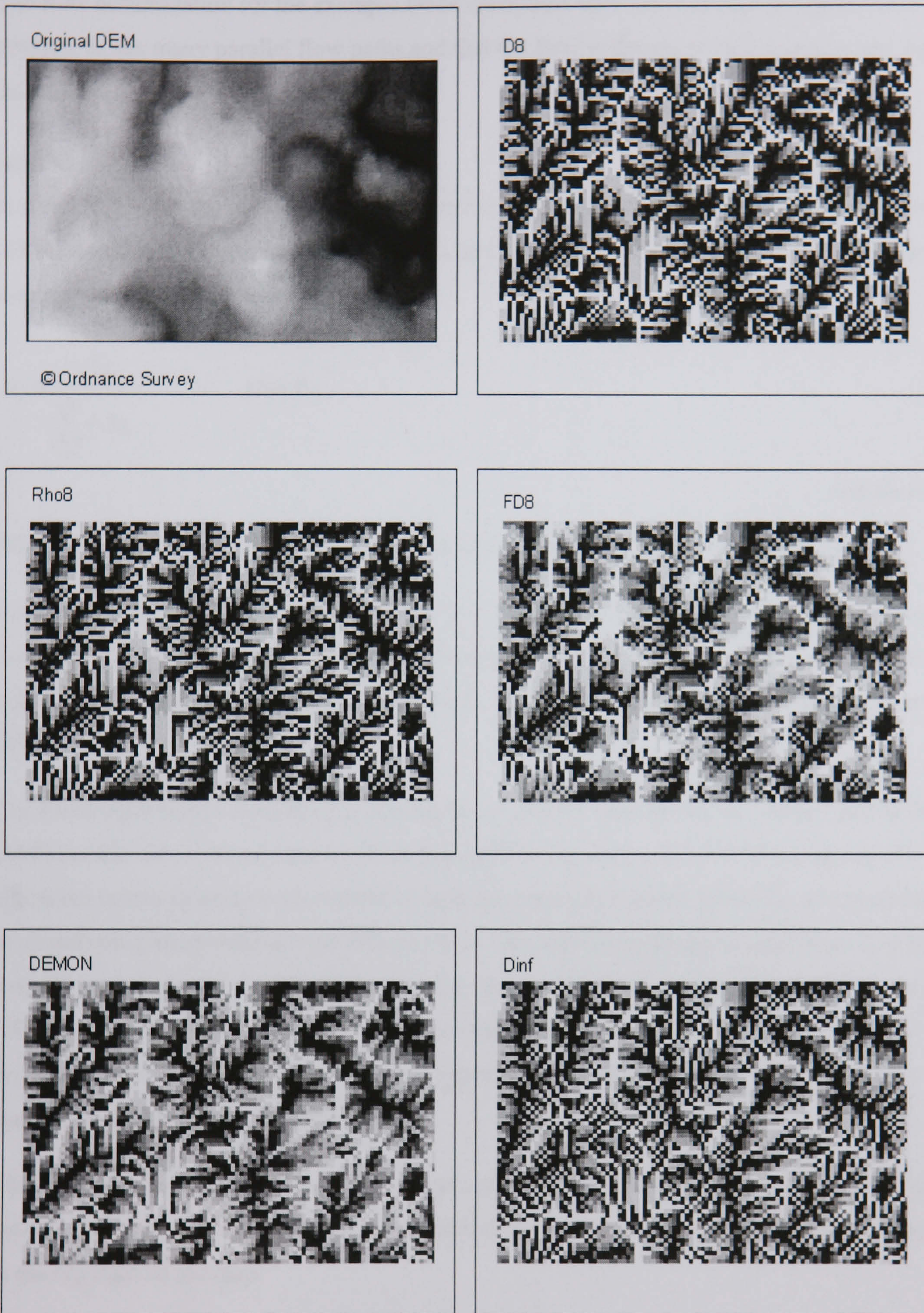
Figure 5.3 Differences in flow accumulation for the different flow direction algorithms
