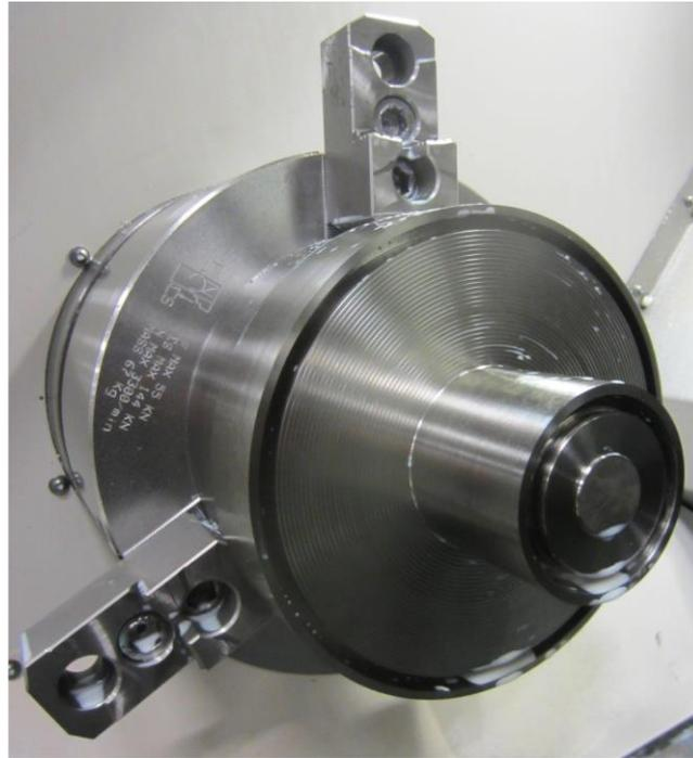
Figure 6.3 Ti-54M billet position held in a MAG Cincinnati Hawk lathe prepared for an orthogonal cutting trial.
