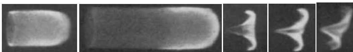
Figure 4.5 Photographs of flame shape propagation down the tube at close both ends
