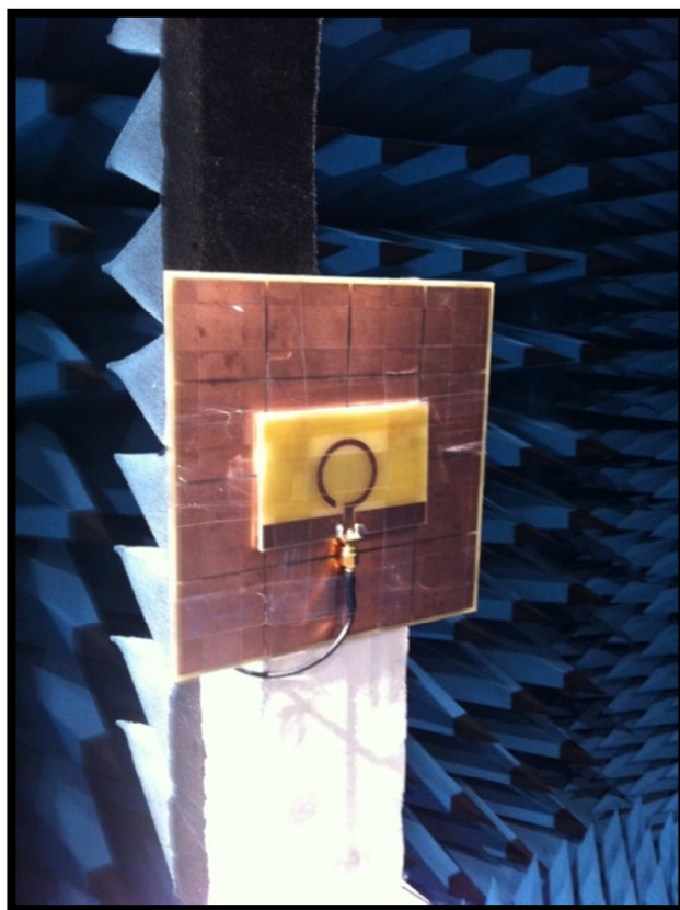
Figure 3.2.22: Fabricated CPW-fed open loop antenna on a square AMC in the anechoic chamber
