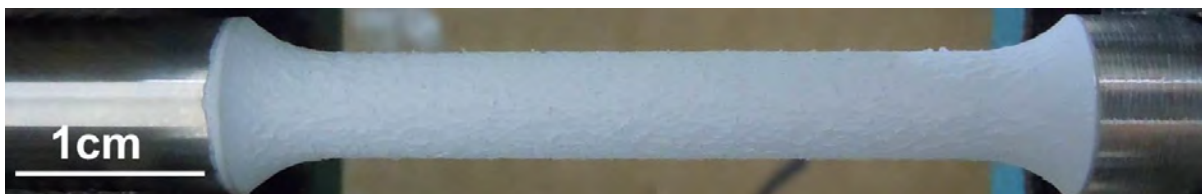
Figure 9-6 Surface of the PEO coated cp magnesium during the tensile test. (The elongation is 7.5%)
