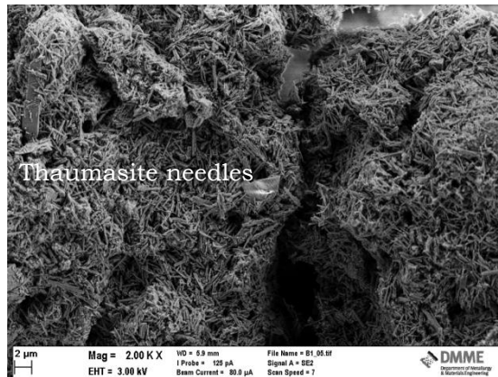
Figure 4.40. Morphology of degraded surface of CEMI-LF mortar stored 360 days in sulfate only solution at 5°C.
