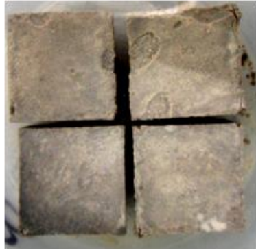
Figure 4.1. 20mm mortar cubes of CEMI-LF mortar stored for 74 days in SC5 at 5°C.
