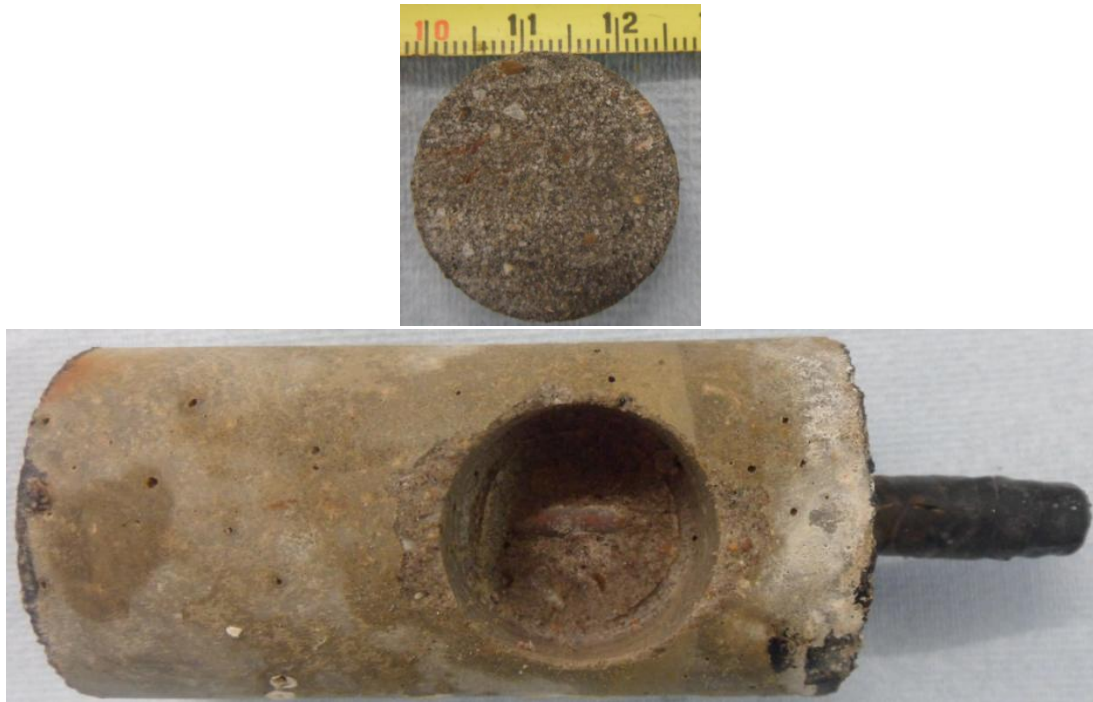
Figure 5.6. Drilled core for permeability test after 900 days of exposure.
