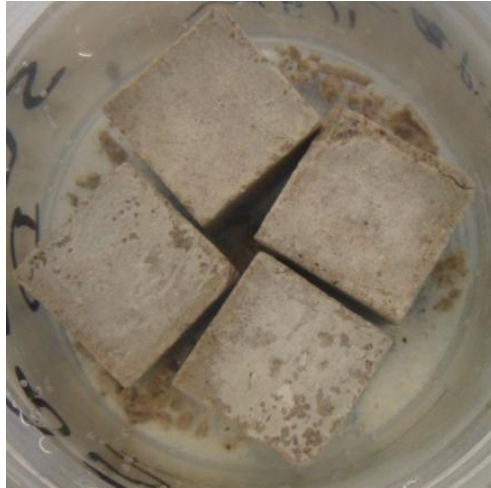
Figure 4.6. 20mm CEMI-GGBS mortar cubes stored for 180 days in SC5 at 5°C.
