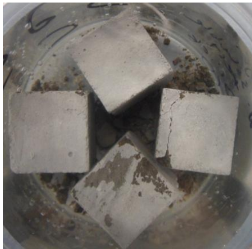
Figure 4.5. 20 mm CEMI-PFA mortar cubes stored for 180 days in S at 5°C.
