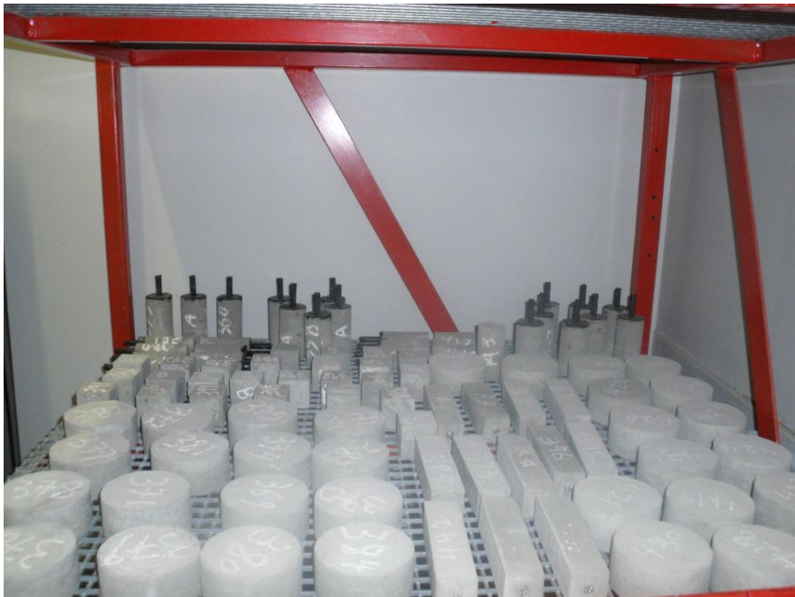
Figure 3.2. Mortar specimens in air curing (~20°C-room temperature).
