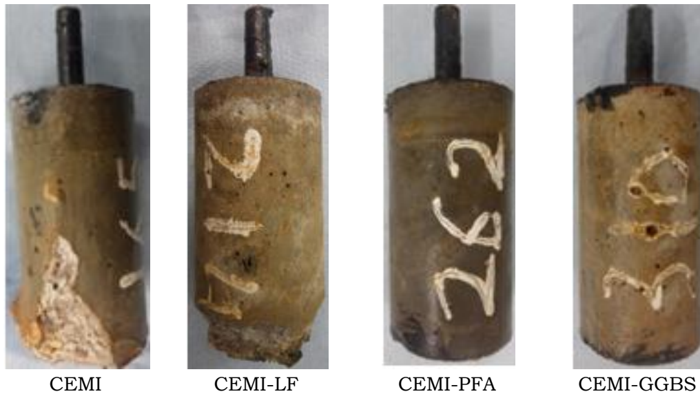
Figure 5.1. Mortar specimens stored for 900 days in SC5 at 5°C.
