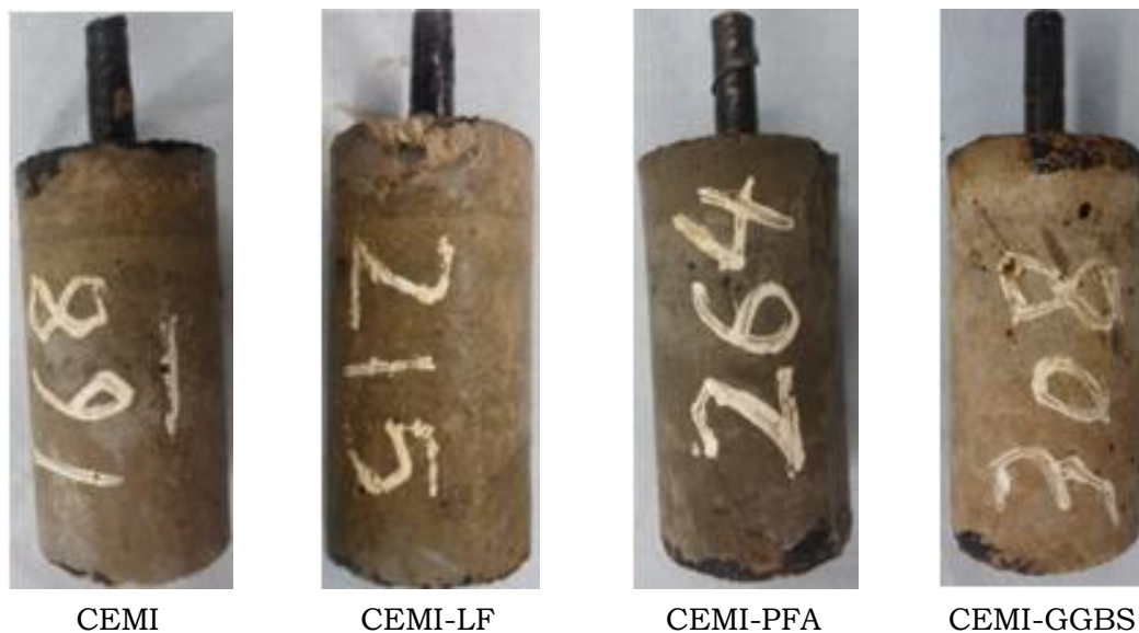
Figure 5.2. Mortar specimens stored 900 days in SC5 at 20°C.
