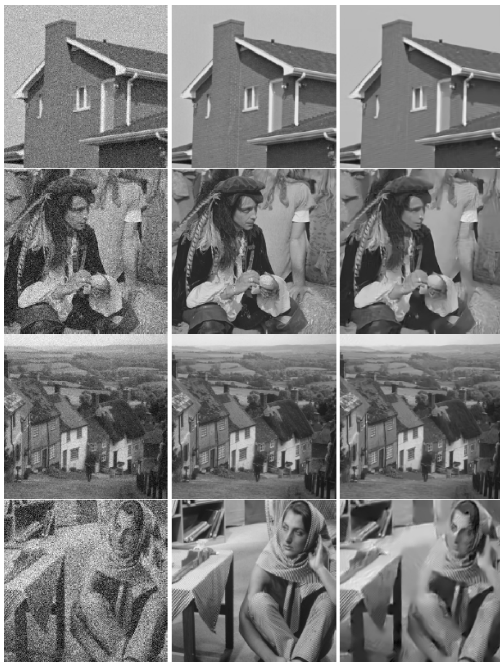
Figure 1.1: The results of image denoising in Mairal et al. 's work (1). Left: noisy images. Middle: original images. Right: restored images. From top to bottom: house ( \sigma = 15 ), man image ( \sigma = 50 ), hill image ( \sigma = 50 ), barbara ( \sigma = 100 ). This figure is borrowed from (2), with the courtesy of Dr. Julien Mairal.
