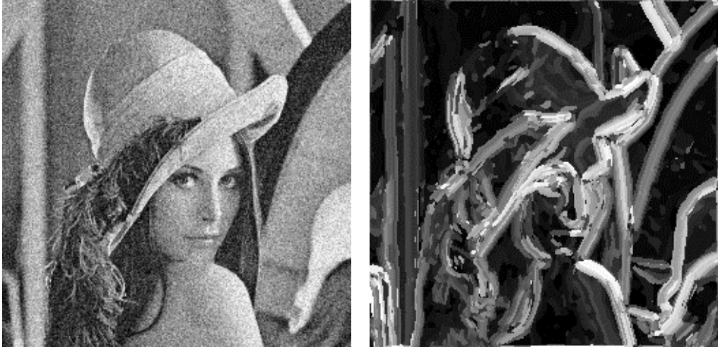
Figure 3.5: The clustering results. Different classes have been represented in different grayscales. The grayscale level [0,255] has been divided by K , and each class k is represented by k \times (255/K) . In this figure, the K is 256.
