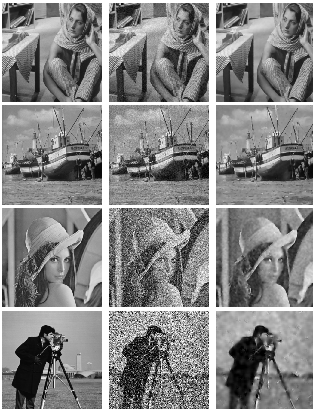
Figure 1.2: The denoising results of KSVD. From top to bottom, the noise levels are: \sigma = 15 , \sigma = 20 , \sigma = 75 , \sigma = 100 .
