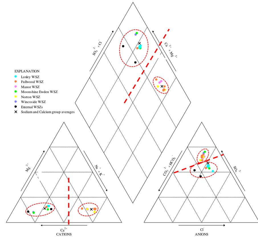
**Figure 25** Piper Diagram of the tapwater characterisation, showing two clusters of tapwater types based on Water Supply Zone (WSZ).
