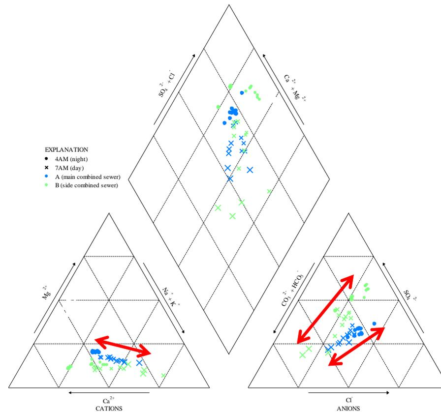
**Figure 30** Piper Diagram for site BS, showing clustering between the two sample points and a spread from night-time to daytime water types. No discernible mixing line is clearly evident.
