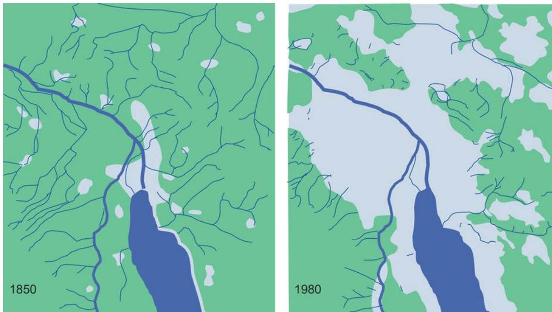
**Figure 5** Historic loss of Zurich's streams (water in blue) with increasing urbanisation (grey). Many streams now flow in culverts, or are diverted into combined sewers. Since 1980, 20 km of streams have been daylighted, with plans for many more (ERZ 2000, 2007). (Image courtesy of Markus Antener, ERZ).
