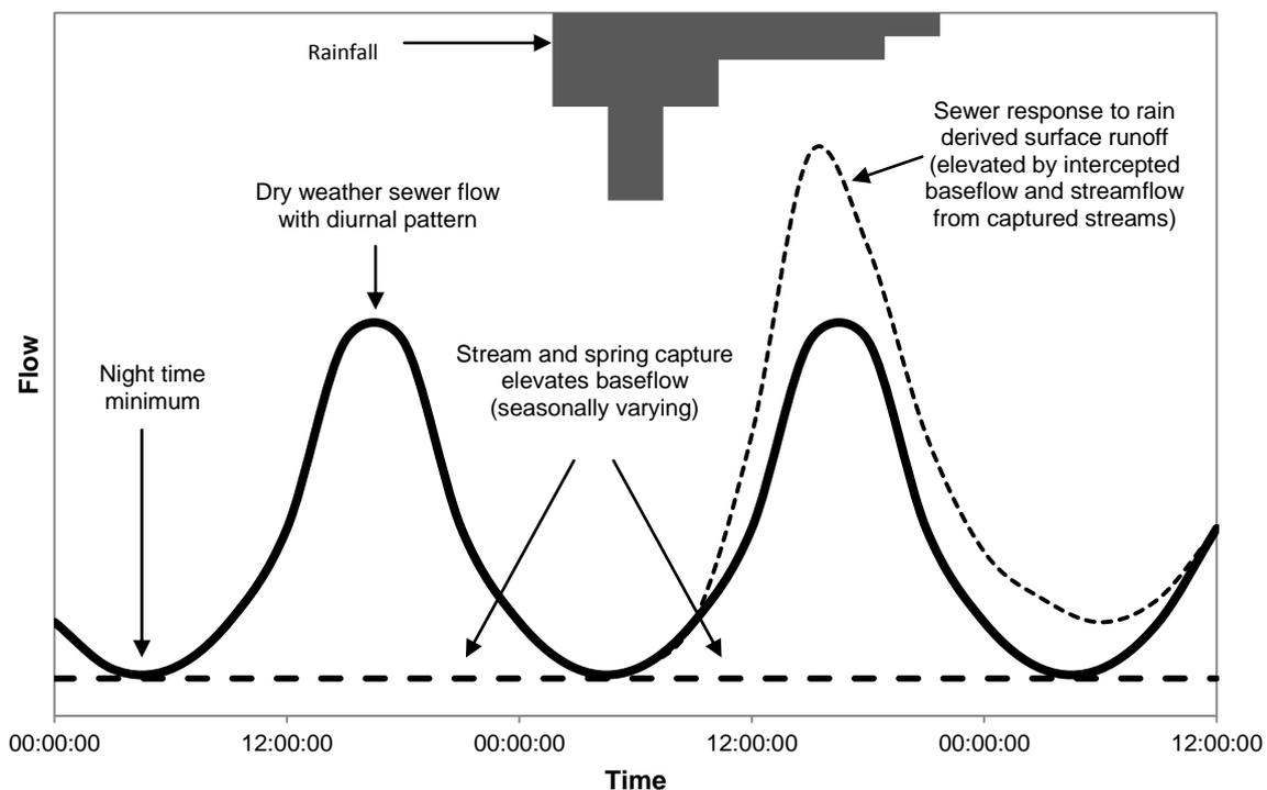
**Figure 3** Idealised unit hydrograph of combined sewer flow and the effects of captured streams and springs on baseflow and surface runoff response.
