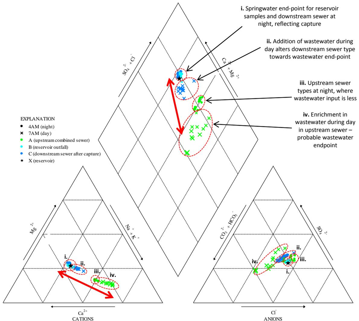
**Figure 26** Piper Diagram for site CV showing distinctive clustering of water types. The upstream sewer sample points are a different water type to the samples from the reservoir outfall. The water types of the downstream sewer lie on a mixing line between the two end-points, trending towards the wastewater end-point during the daytime samples, and being essentially the same as the captured water end-point during the night-time.
