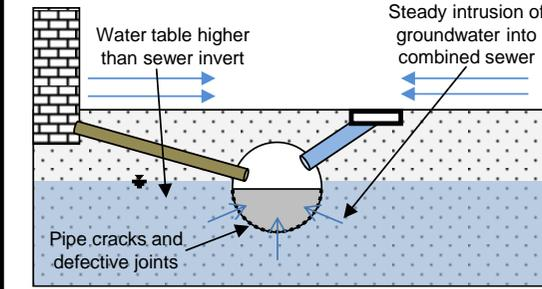
1. Modern situation: unintentional leakage of groundwater into combined sewer through pipe cracks and defective joints.
