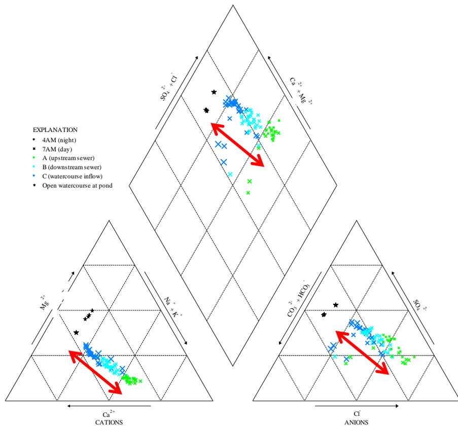
**Figure 27** Piper Diagram for site PW showing distinctive clustering of water types. Samples lie on a mixing line between the open watercourse end-point and an end-point of the upstream sewer. The downstream sewer samples lie on this mixing line, trending towards the watercourse end-point at night.
