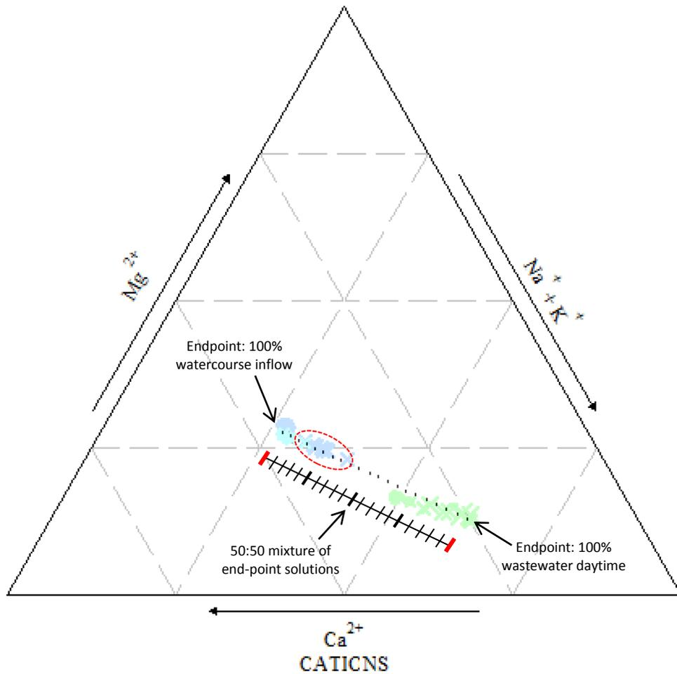
**Figure 31** Quantification of proportions of captured flow in the downstream sewer (C) at site CV. Simple mixing of end-point solutions was calculated at different ratios to quantify the cation mixing line, plotted alongside, showing non-linearity of scale, in order to read off the range of proportions where the downstream sewer sample cluster lies (circled).
