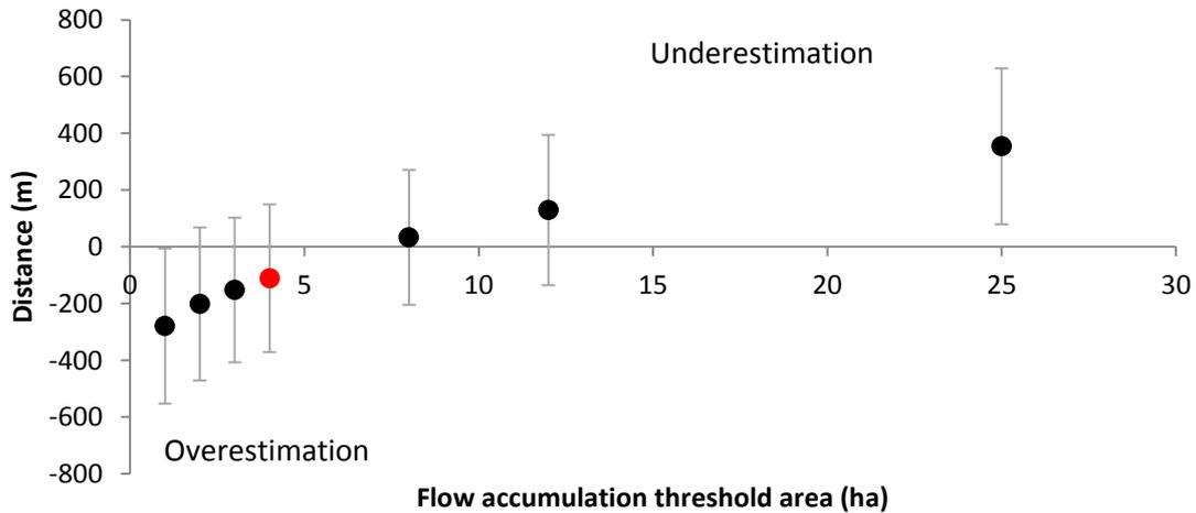
**Figure 9** Topographic flowpath training results showing the average distance (with error bars showing standard deviations) between the modelled topographic flowpath stream origins and training points, for seven flow accumulation thresholds as upstream contributing areas. Chosen threshold of 4 ha (i.e. 400 cells) in red.
