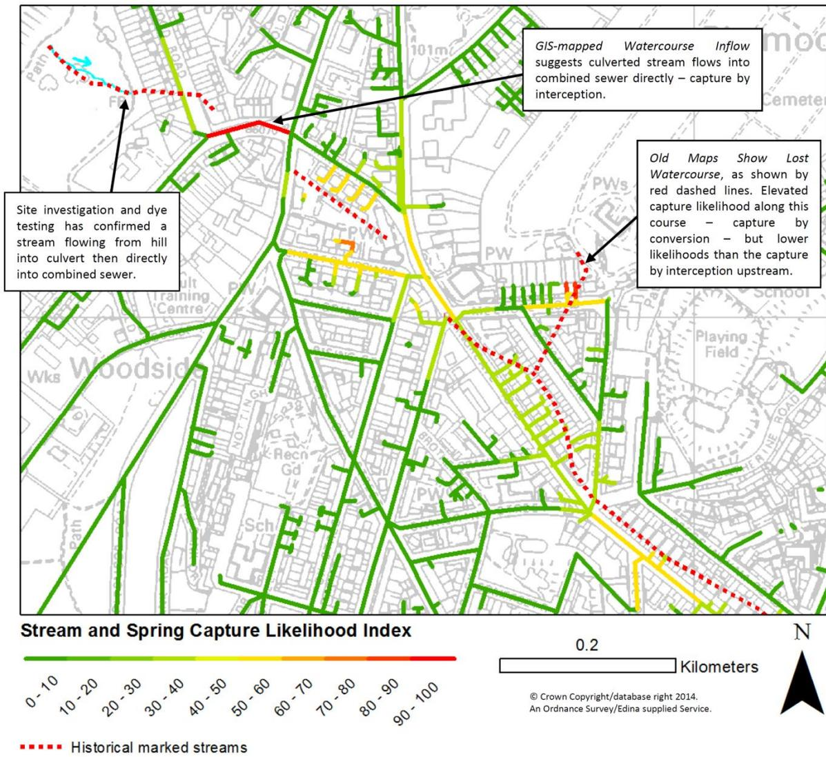
**Figure 39** Correctly predicted stream and spring capture at one site, where a watercourse is known to flow into a combined sewer. Combined sewers are colour coded by the Stream and Spring Capture Likelihood Index, which also picks up elevated capture likelihood along the route of an historic stream shown on old maps (dashed red).
