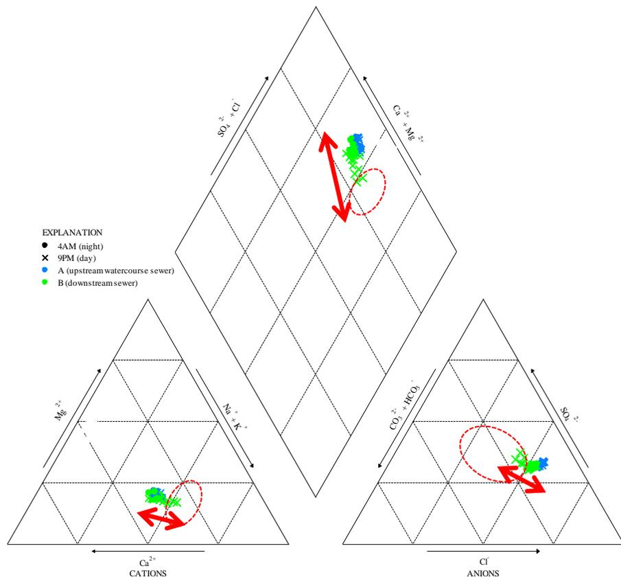
**Figure 29** Piper Diagram for site HB showing distinctive but very similar clustering differentiating the captured water and the downstream sewer. Daytime sewer samples trend towards a hypothesised wastewater end-point, away from the captured water type.
