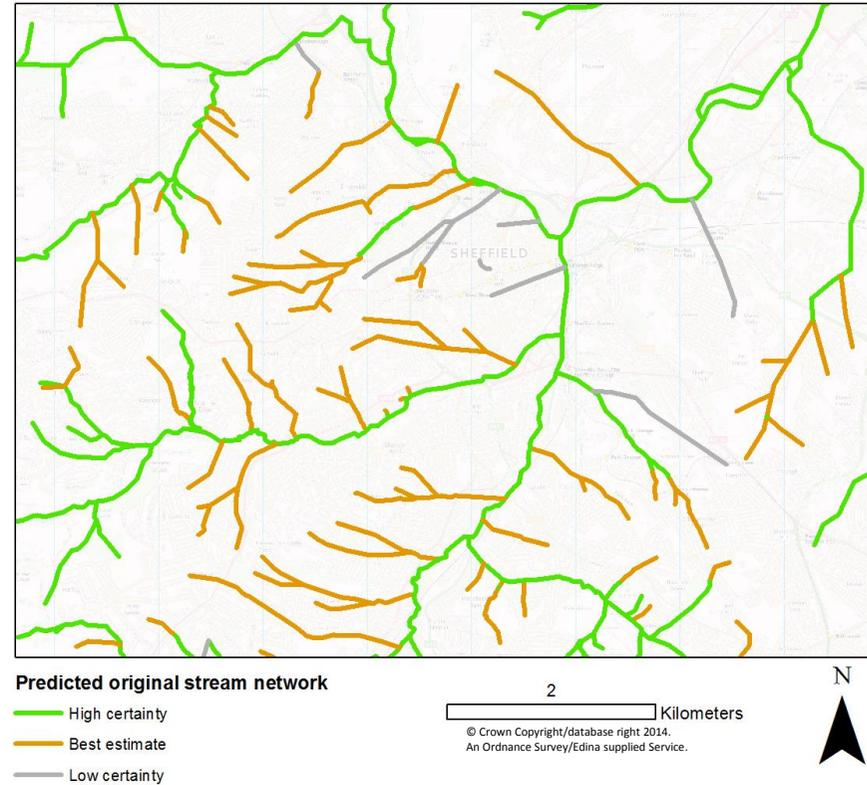
**Figure 13** All lines of evidence visually combined to show full stream network, including both existing and lost streams, and colour-coded to reflect locations of low certainty (conflicting or very sparse evidence) and high certainty (streams or culverts definitely shown on modern maps).
