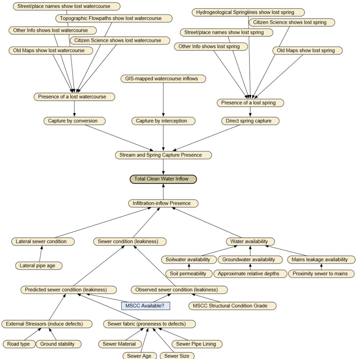
**Figure 34** BBN model structure showing the variables and their relationships (shown as nodes and links between the nodes). Variable states are detailed further in **Table 16**.
