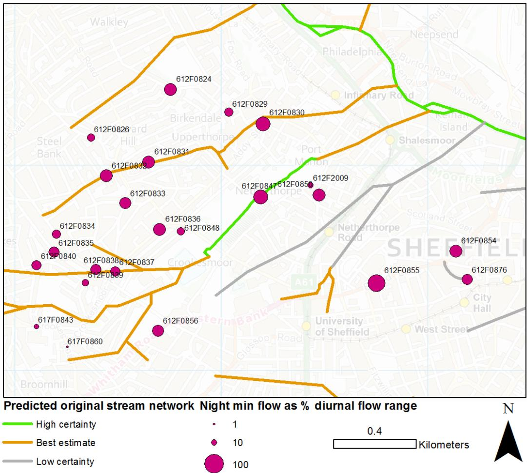
**Figure 51** Sewer flow monitor locations (shown scaled as night time minimum flow as % of diurnal flow range) compared with the locations of lost streams in the area.
