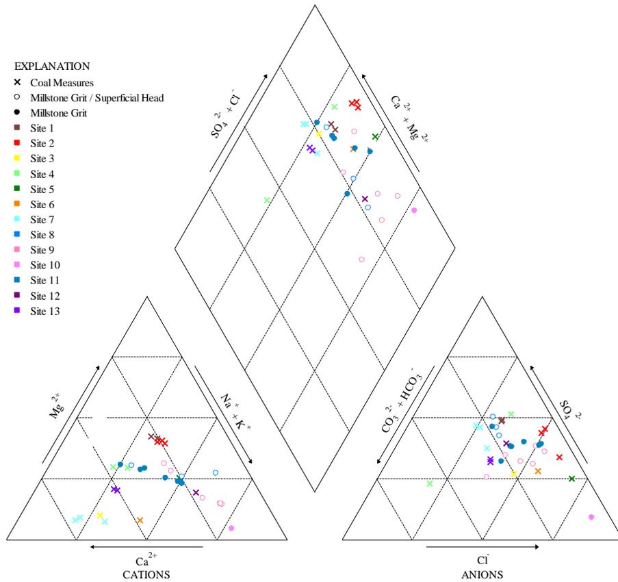
**Figure 24** Piper Diagram of the springwater characterisation, showing no clearly discernible water type groups based on underlying geology. Even samples at the same site can be highly variable in water type.
