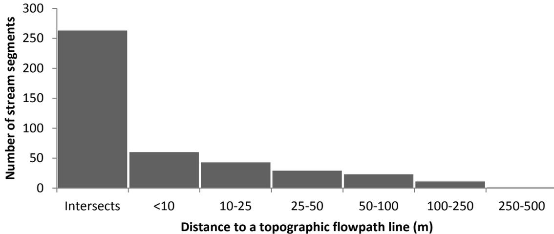
**Figure 14** Histogram showing distances of each stream segment marked on historical maps to the nearest topographic flowpath line. The majority touch or intersect the nearest topographic flowpath line.
