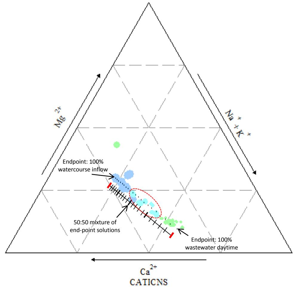
**Figure 32** Quantification of proportions of captured flow in the downstream sewer (B) at site PW. Simple mixing of end-point solutions was calculated at different ratios to quantify the cation mixing line, plotted alongside, showing non-linearity of scale, in order to read off the range of proportions where the downstream sewer sample cluster lies (circled).
