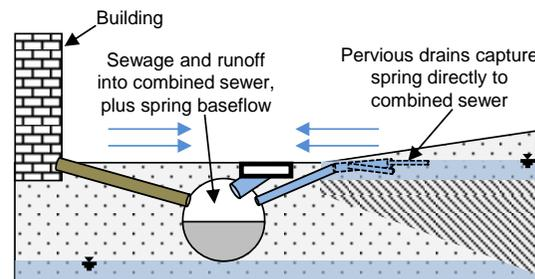
2. Modern situation: spring deliberately drained into combined sewer to enable development.
