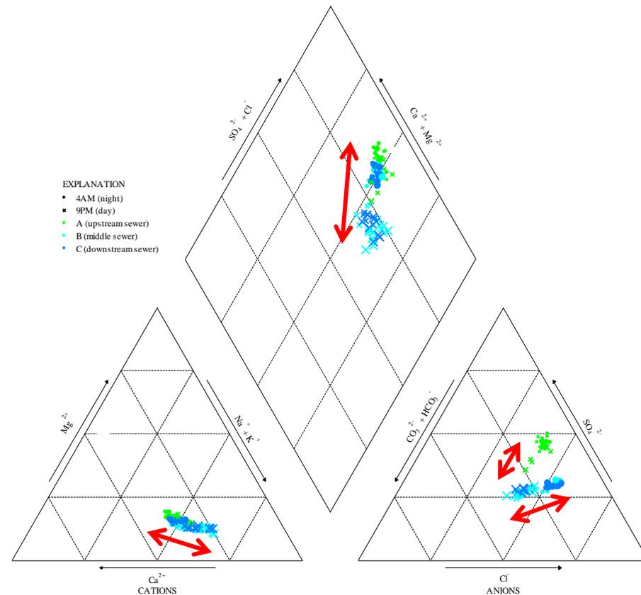
**Figure 28** Piper Diagram for site SR showing distinctive clustering of water types, most clearly differentiated by anions, which show the upstream sewer to be of different water type to the middle and downstream sewers, though neither grouping appear to correspond with local springwaters.
