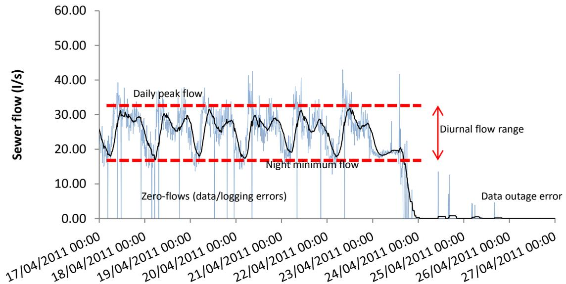
**Figure 52** Night time minimum flow analysis illustrated for sewer flow monitor F0831, showing the flow time-series with a 24 point moving pass filter that reduces the high frequency noise to extract the diurnal pattern. Night minimum flow and daily peak flow lines are visually fitted, and the night minimum flow as a % of the diurnal flow range is calculated.
