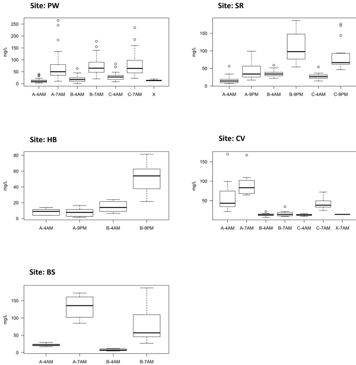
**Figure 33** Boxplots showing COD (mg/L) concentrations for each site, by sample point and time period. COD in sewers is significantly higher during the daytime samples than at the night-time minimum. Watercourse samples do not significantly vary day and night, as expected. The exception is at site PW, where the COD at the watercourse inflow (C) is elevated during the daytime – evidence of contamination by misconnections.
