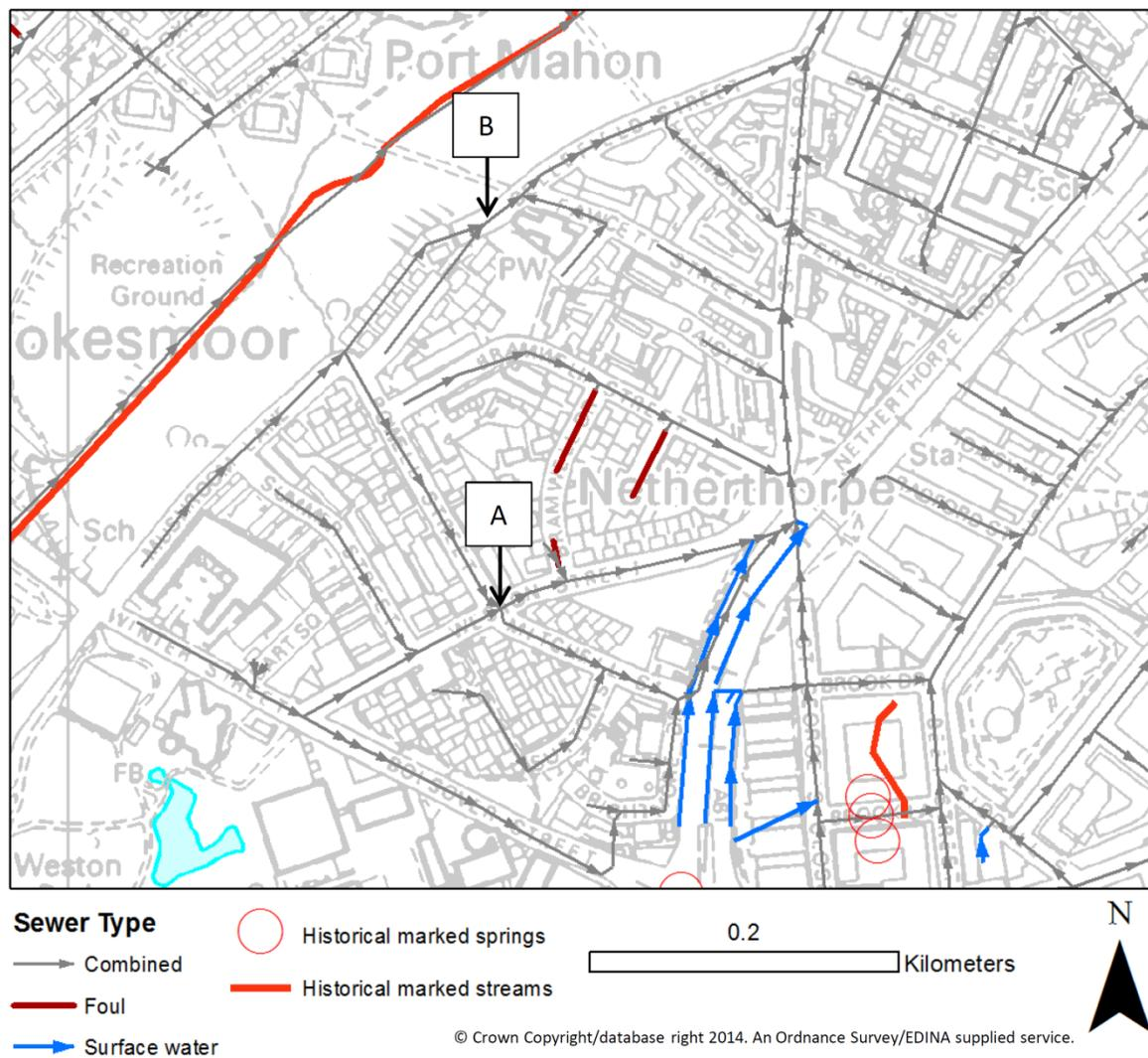
**Figure 22** Sewer capture sample location map and pictures for site BS. Despite some possible lost streams in the area, there is no evidence of capture. A – main combined sewer, larger wastewater catchment displaying elevated night-time minimum flow according to flow data. B – side combined sewer, smaller receiving catchment.
