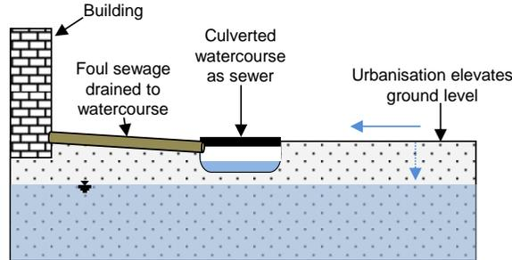
2. Early development: watercourse receives surface runoff and foul sewage, and is covered (culverted) to sanitise.
