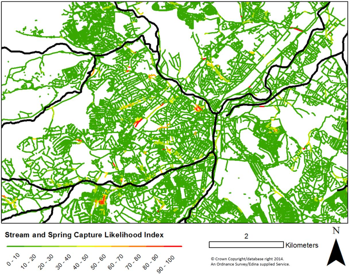
**Figure 37** Sheffield combined sewer network colour-coded by stream and spring capture likelihood index. The river and canal network are outlined in black for reference.
