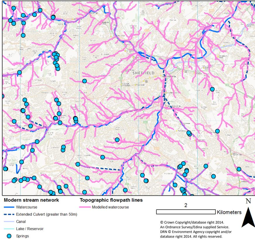
**Figure 12** Topographic flowpath lines, with modern stream network and springs.
