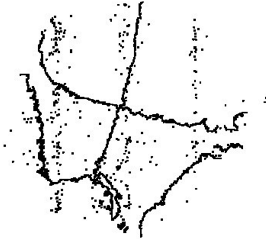
Figure 78 EBSD grain boundary misorientation map obtained from the sample shown in Figure 76 where misorientations of > 10\% are plotted.
