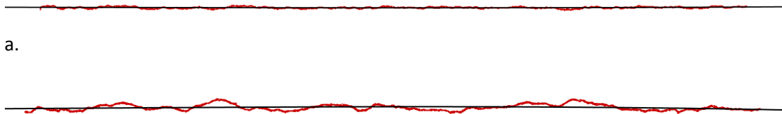
b. Figure 3.29 Specimen spiral - a. Path width measurements (red) and trendline. b. Spacing measurements and trendline. The specimen spiral had path width trend parameters of 0,0,0 and spacing trend parameters of 0,0,0.01.
