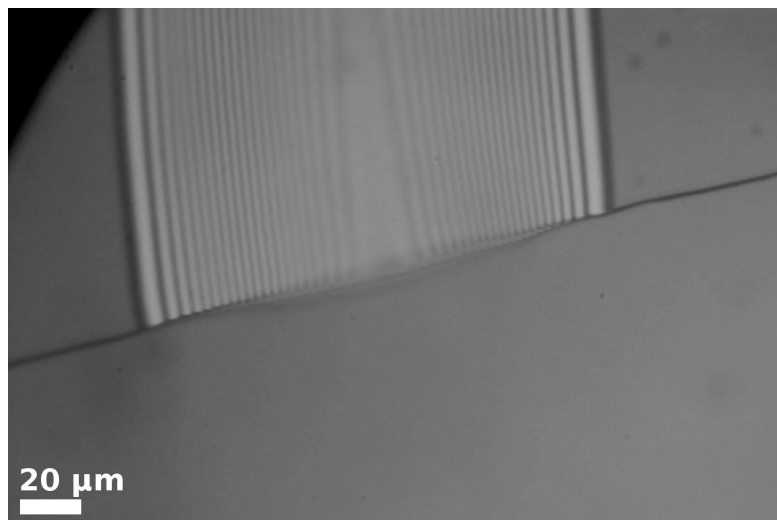
FIGURE 6.7: Optical micrograph of a mica pocket opening viewed in narrow bandwidth 532 nm light. The first fringe is dark, in direct contradiction to Equation 6.1.
