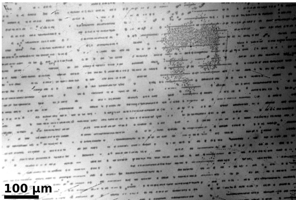
FIGURE 4.22: Optical micrograph showing ice grown on ion-milled silicon.
