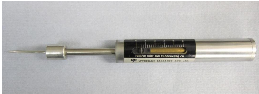
Figure 3.7: Modified penetrometer fitted with a thick needle attached to plunger
