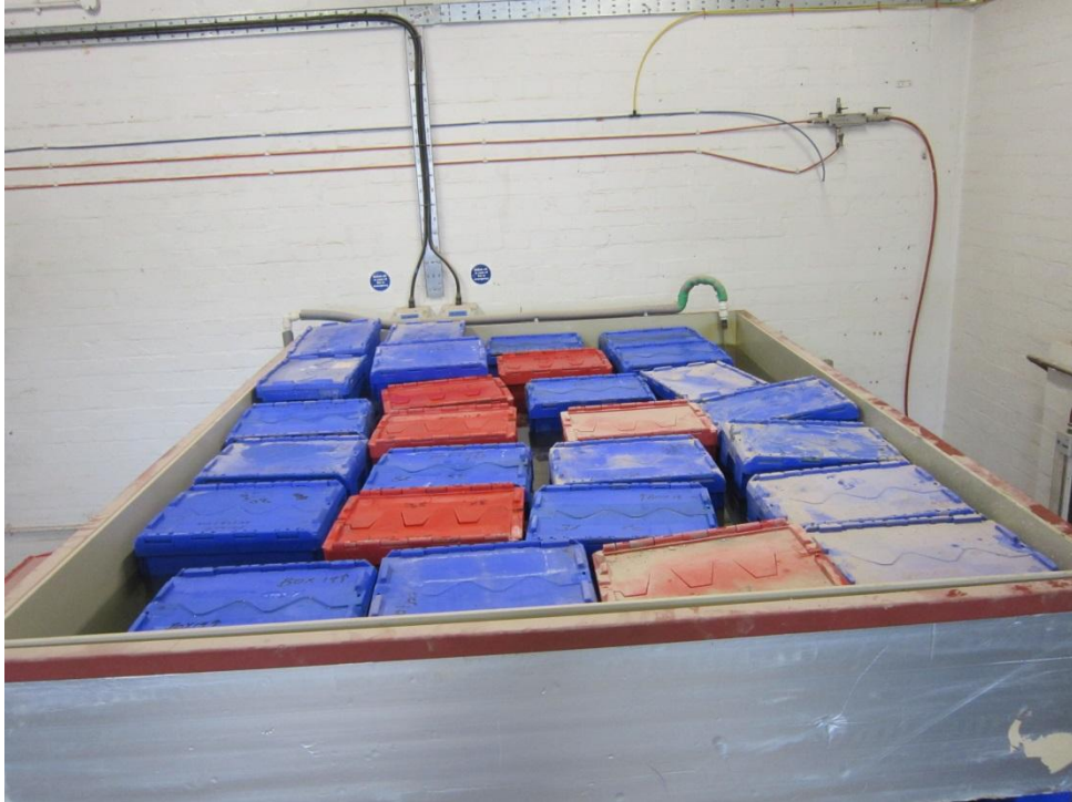
Figure 3.5 the long –term curing in tanks
