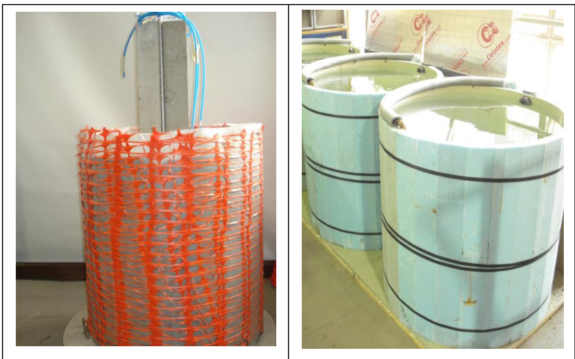
Figure 3.6 Temperature controlled tanks and exposure of concrete to clay
