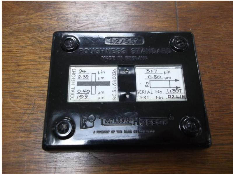
**Figure 3.11.** The calibration standard for the Talysurf. Calibration of the machine with the right hand square is carried out before and after each session to confirm that no damage had taken place to the stylus ensuring correct results are recorded.
