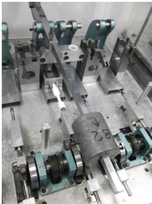
**Figure 3.9. Complete assembly of the six station wear rig.**
