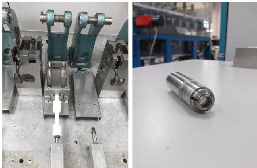
**Figure 3.7. The plate set up and pin holding assembly. A.** The bath well, bath insert and plate were assembled before being placed onto the reciprocating stage. The assembly was then secured with the connecting rod. **B.** The osteochondral pin was placed inside the set up shown with the cartilage surface protruding.
