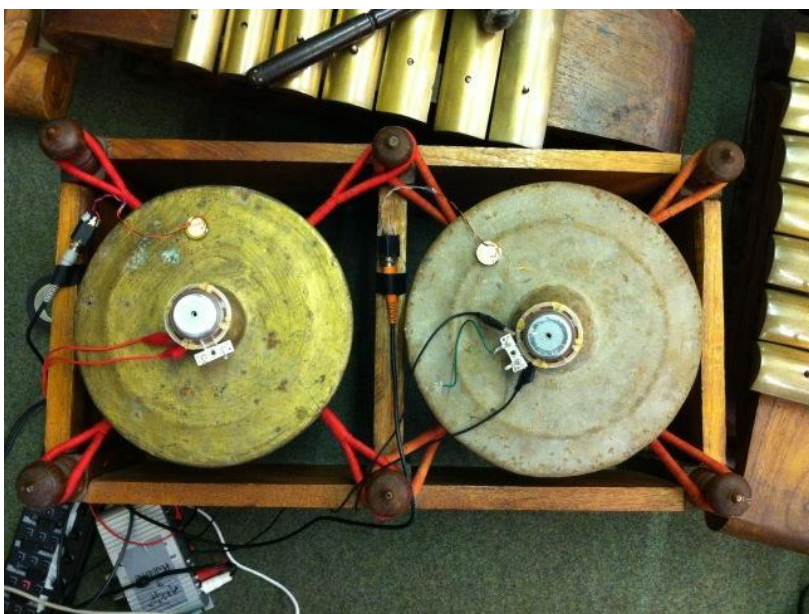
Figure M.1: Augmented Gamelan instruments, with transducers and piezoelectric microphones attached
