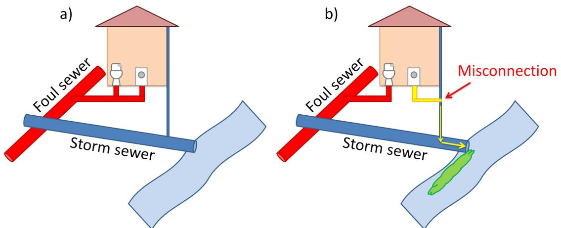
Figure 2.1: a) Correctly connected separate sewer system. b) misconnected separate sewer system
