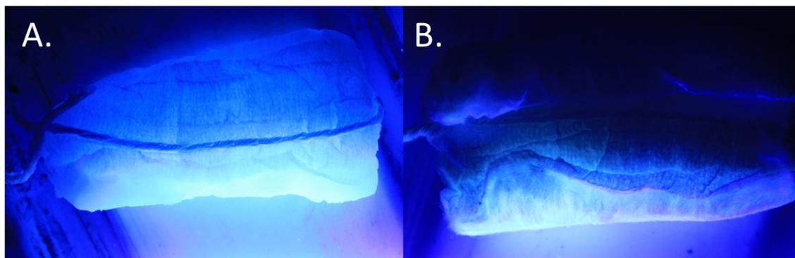
Figure 3.2: Samplers exposed to UV light to show fluorescence. A. Fluorescing tampon sampler. B. Tampon sampler showing reflection of UV light, but no fluorescence.
