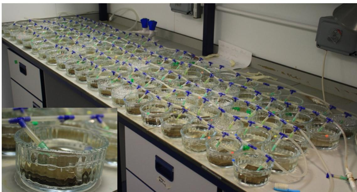
Figure 4.1: Microcosms containing algal communities on tiles, nutrient solutions and artificial detergent effluents, aerated using needles connected to air supply. Inset closer picture of microcosm
