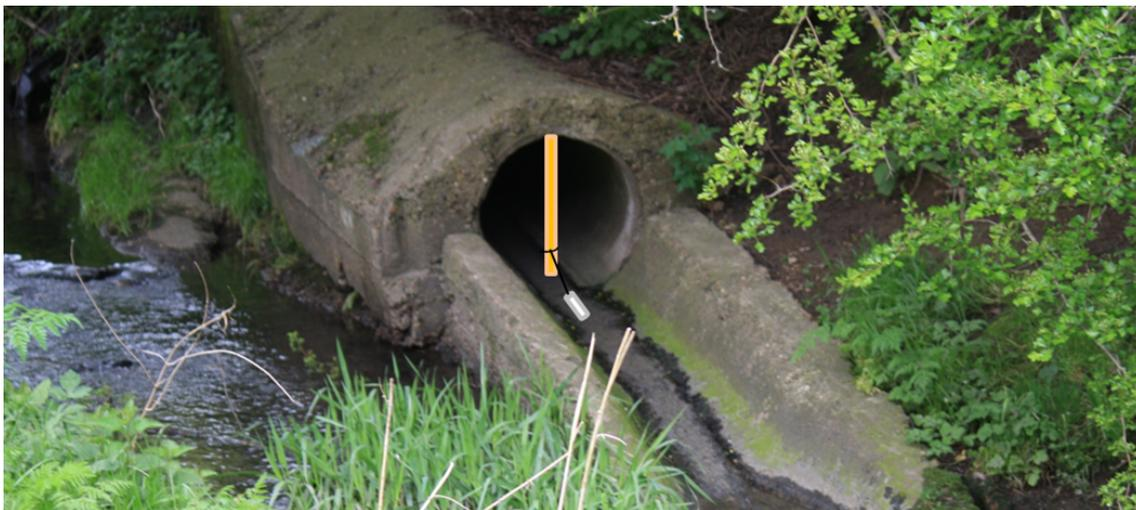
Figure 3.1: A representation of a passive OB sampler consisting of a tampon tied to a length of bamboo cane, in situ at a surface water outfall.
