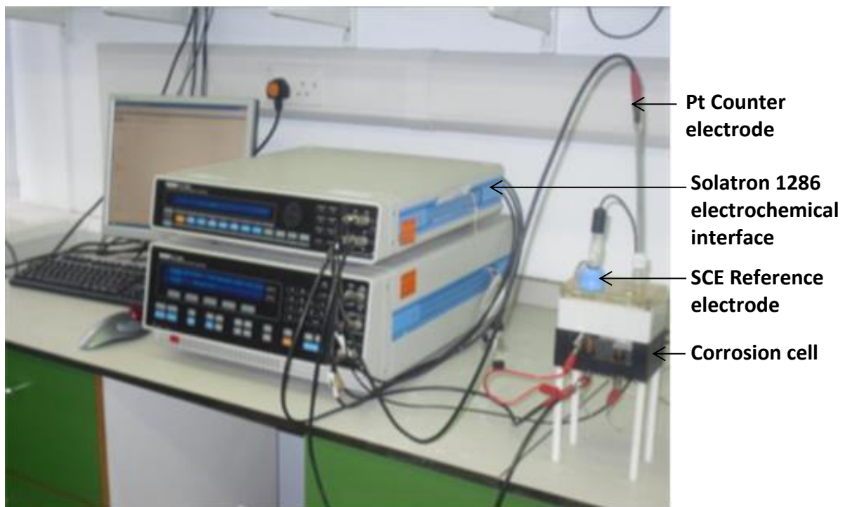
Figure 3.7: Experimental arrangement for making potential measurement.
