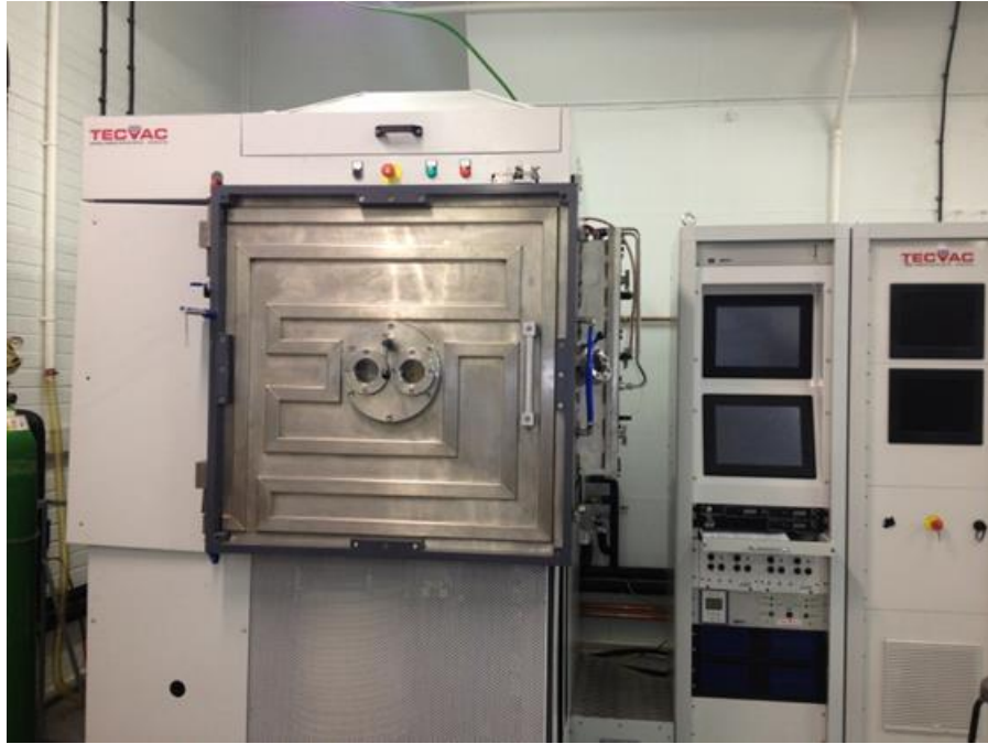
Figure 2.6: EBPVD deposition equipment.
