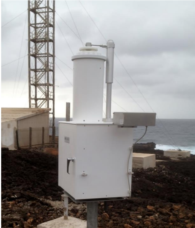
Fig 10. Wet precipitation collector for analysis of mercury content in precipitation samples installed in July 2014
