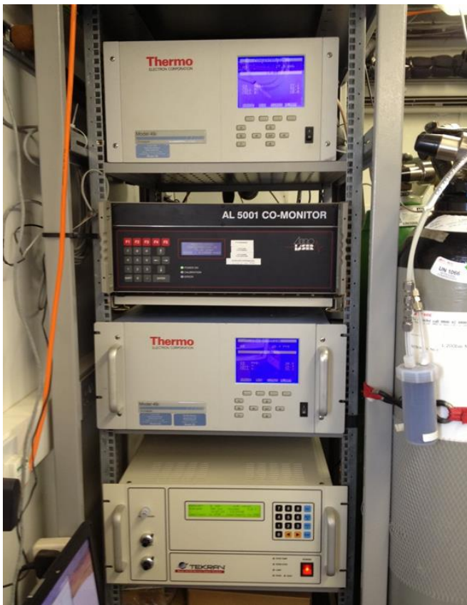
Figure 9. Analyzers for continuous measuring of Ozone ( O_3 ), Carbon monoxide (CO) and total gaseous mercury (TGM) at the Cape Verde Atmospheric Observatory - CVAO
