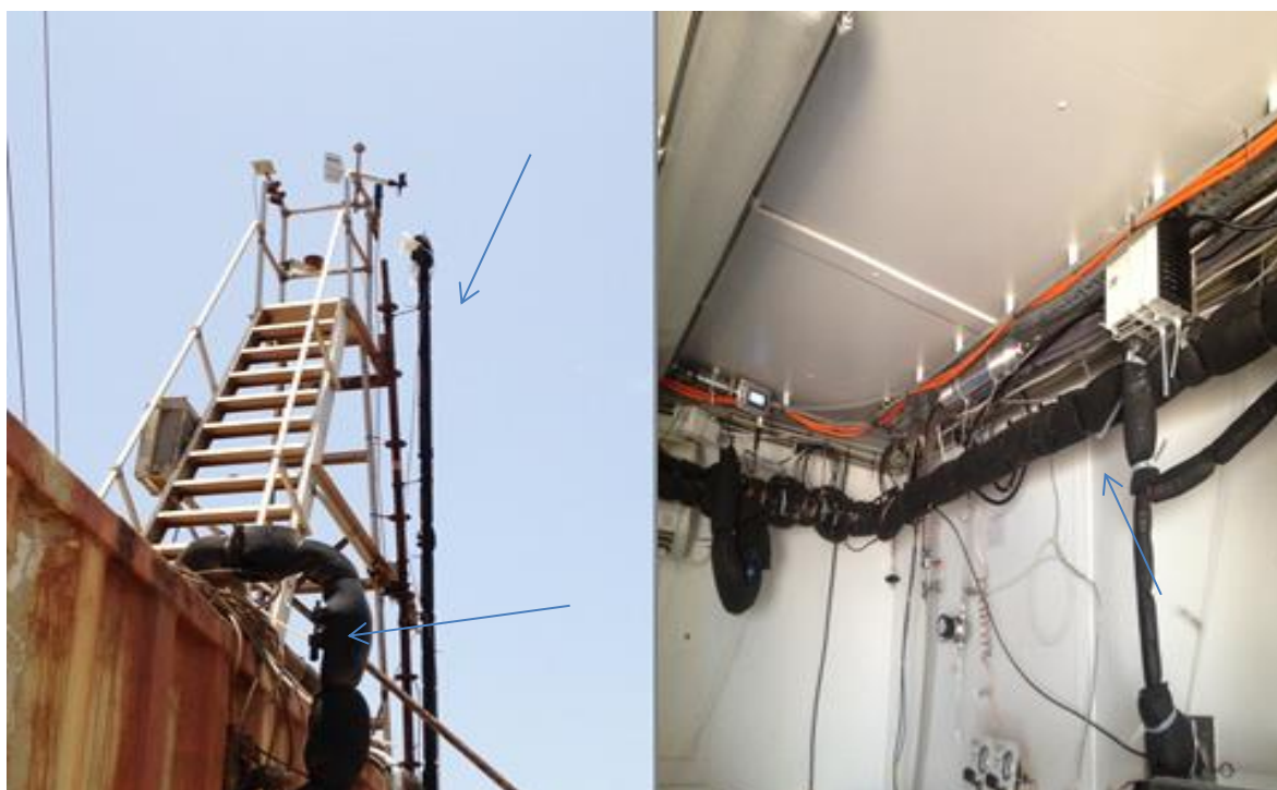
Figure 11. Photo shows the glass inlet line from 10 meter sampling tower and pathway into the laboratory.
