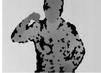
Figure 2.7: Noise in depth image.
