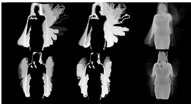
Figure 2.10: Illustration of the MHI , INV and GEI in two tokens (top row and bottom row). The projection images show that MHI emphasizes recent motion, i.e. ending frames whilst INV the beginning frames. GEI encodes the average gait information and is supplementary in repetitive actions where both MHI and INV are poor at representing.
