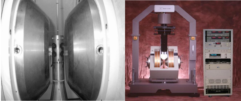
Figure 69: Pick up coil configuration of Microsense Model 10.
