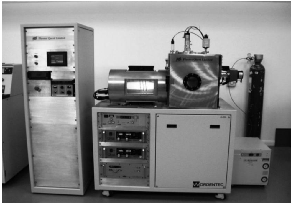
Figure 62: Photo of HiTUS sputtering system.
