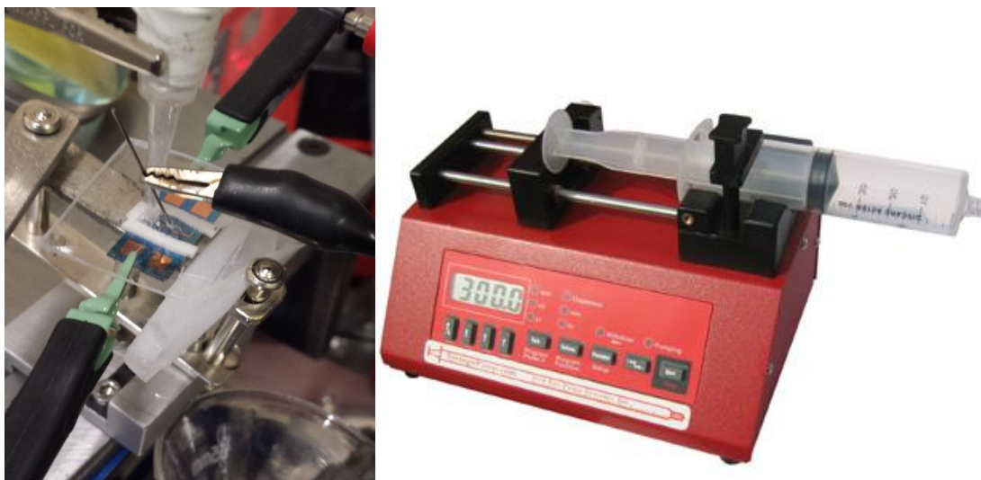
Figure 39, the home- made flow cell (left), and the NE-300 syringe from New Era Pump Systems, Inc. (above).
