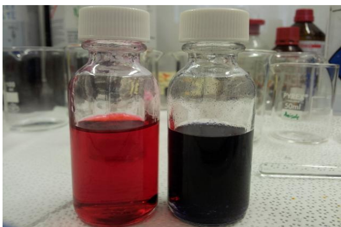
Figure 36, a solution concentration of BBL in MSA about 0.2 mg/ml with red colour (left), and a same concentration of BBL nano- belts after a mixture of Methanol, Chloroform and MSA with dark blue colour (right).
