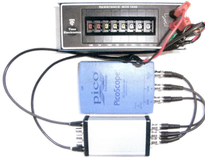
Figure 49, the complete system, from top to bottom, resistance box, Picoscope and characterisation board (I-V converter).
