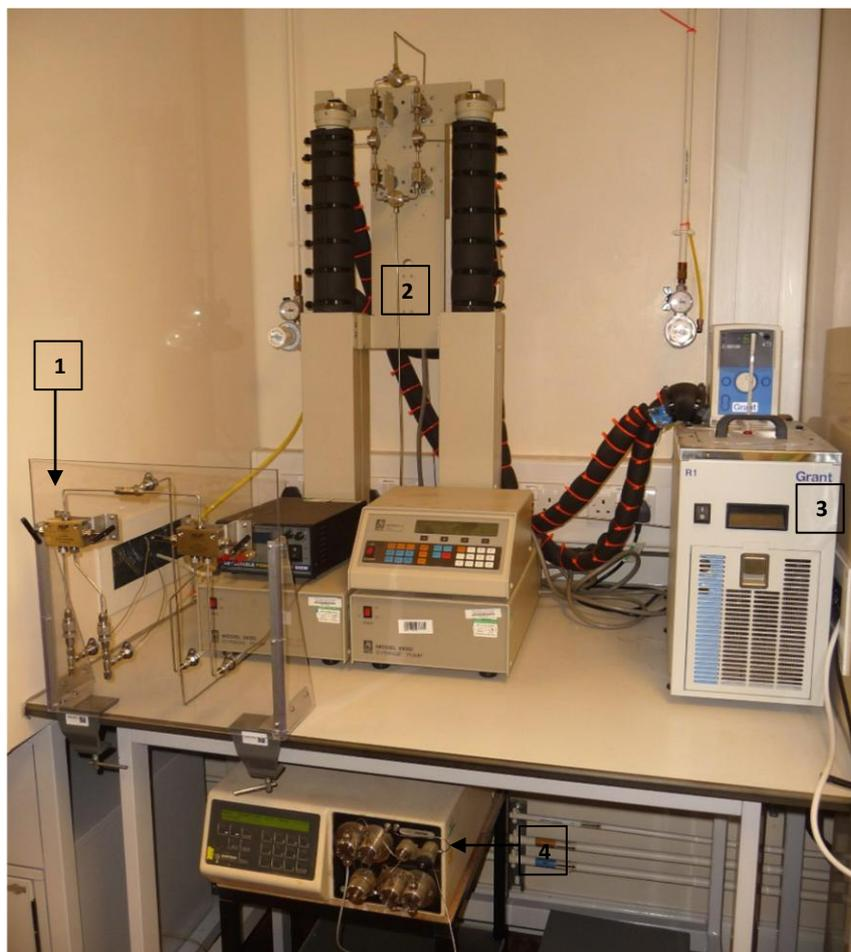
Figure A-I.3. Photo of the high pressure CO<sub>2</sub> supply system. Central control panel (1); high pressure pump (2); chiller (3); HPLC pump (4).
