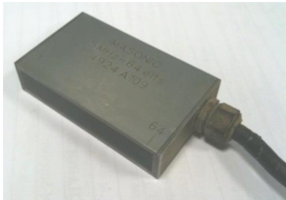
Figure 3-10. A 5 MHz 64 element ultrasonic array transducer.
