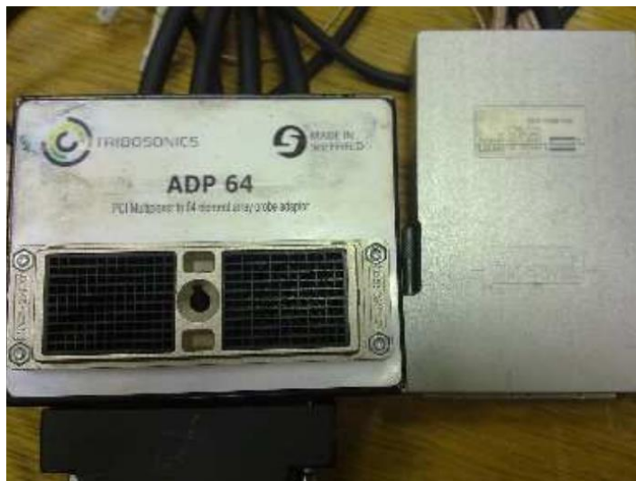
Figure 3-13. Pickering multiplexer connector and the adaptor to fit the array transducer.
