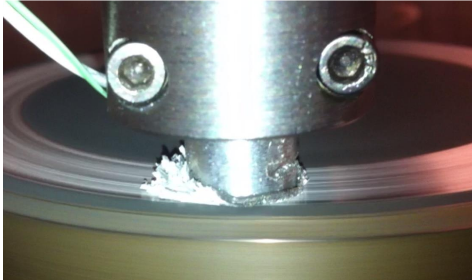
Figure 4-11. The pin and disk mid-test with the pin experiencing a large amount of material displacement.
