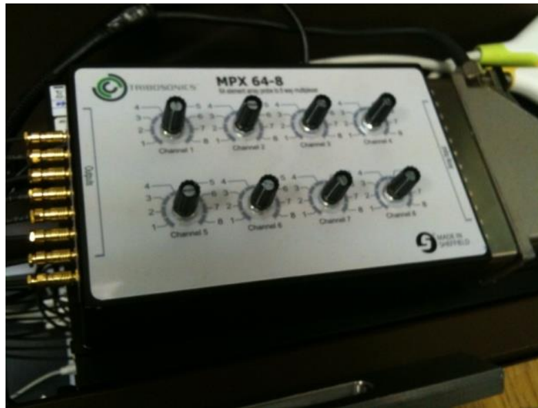
Figure 3-11. The ultrasonic array switching box.
