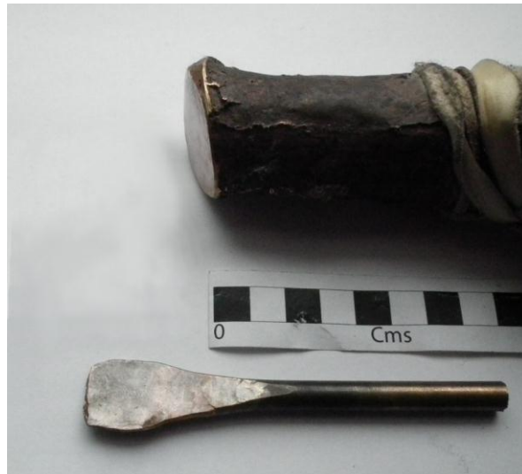
Figure 6.12 Hammer A1 after use with chisel
