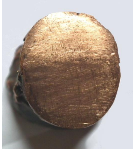
Figure 6.22 Hammer C1 after maintenance
