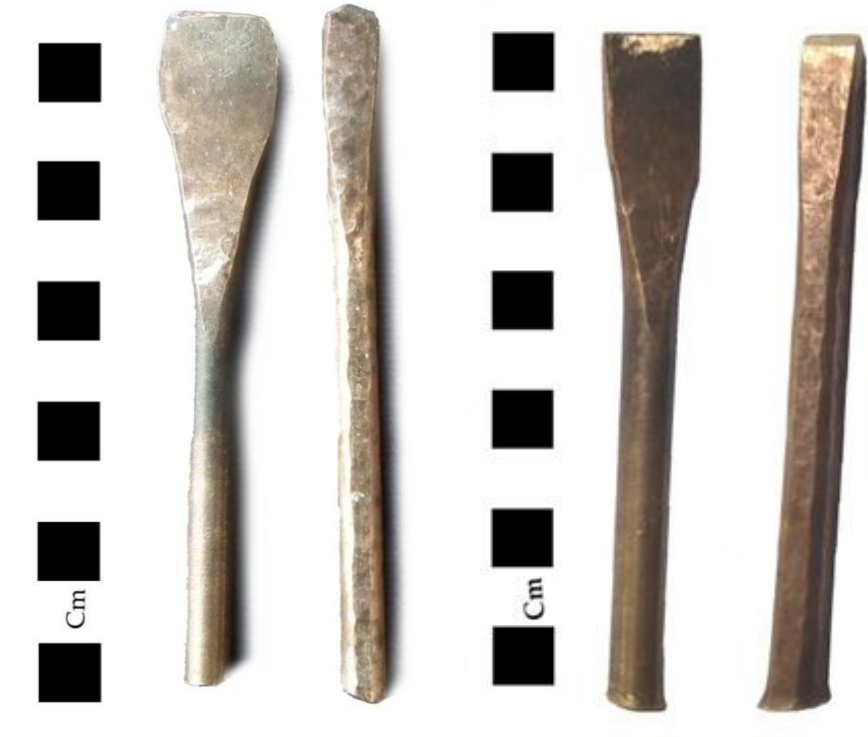
Figure 6.8 Chisels before and after use
