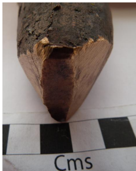
Figure 6.10 Hammer F1 before and after forging. Note flattened apex after use
