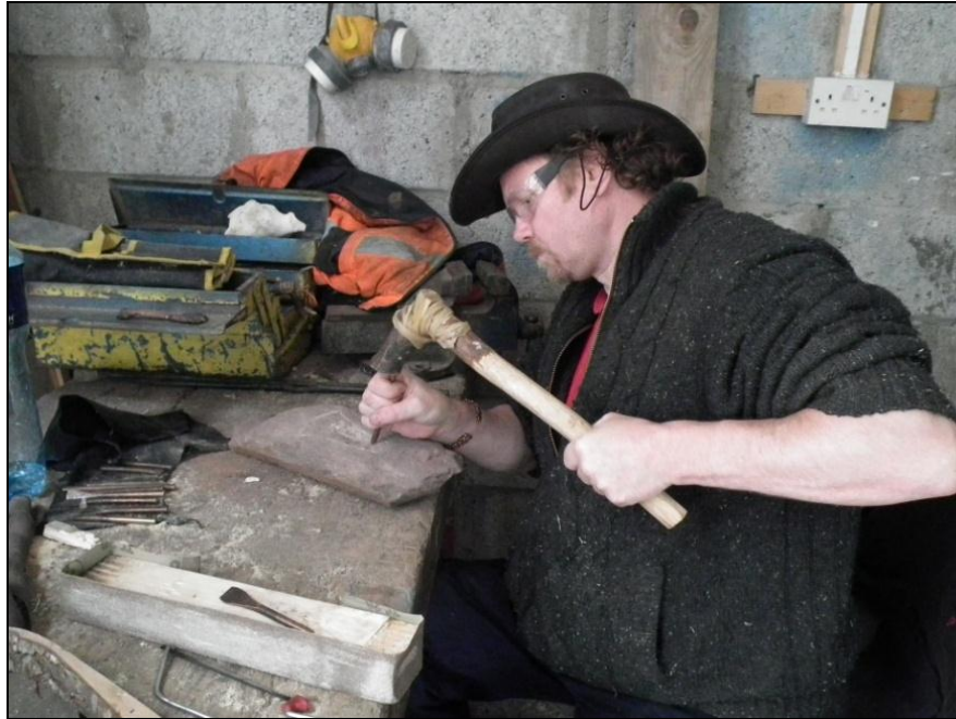
Figure 6.7 Carving the mould
