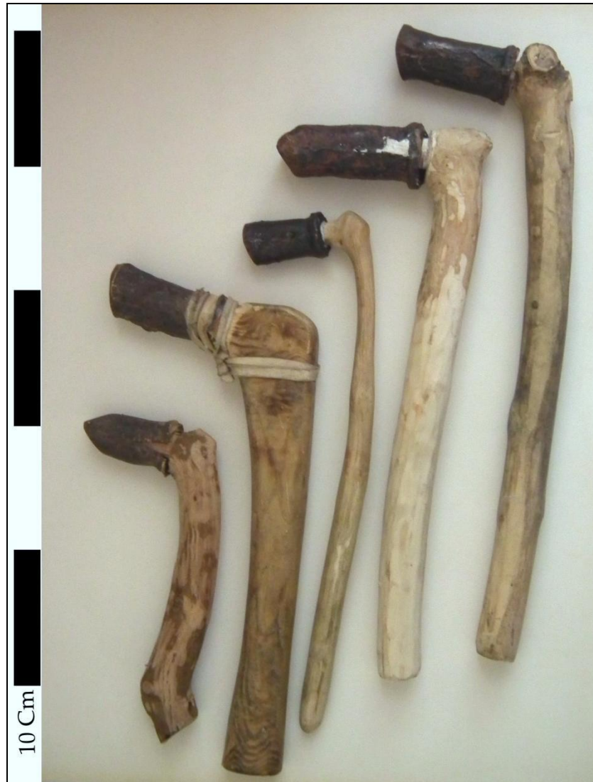
Figure 6.1 Different styles of handles left to right: cherry, oak, cherry, willow, willow
