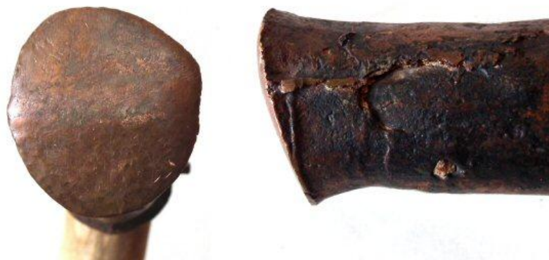
Figure 6.5 Hammer A2 after use
