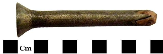
Figure 4.3 Possible rivet snap, British Museum (photo by author © Trustees of the British Museum)
