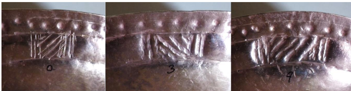
Figure 6.20 Chasing on bowl produced by chisels 0, 3, and 9
