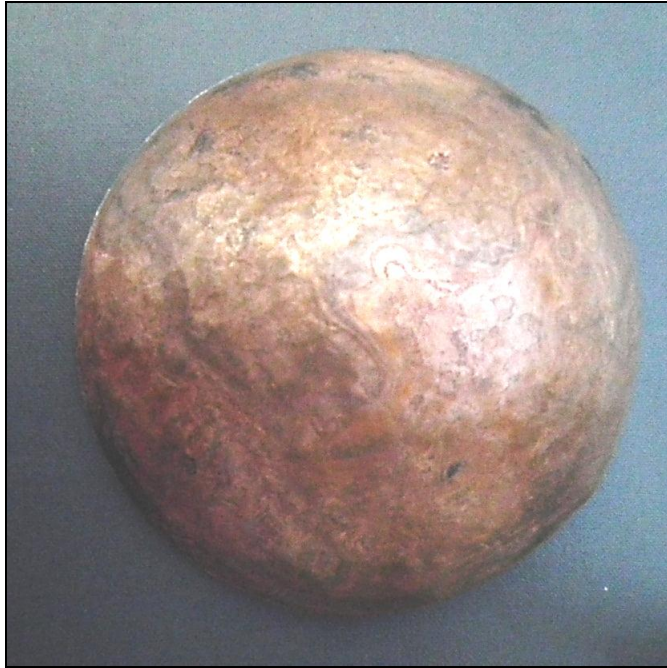
Figure 6.15 Bottom surface of bowl after forming
