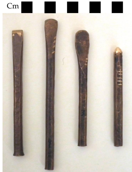
Figure 6.18 Chisels selected as chasing tools: From left to right 0, 9, 3, 5
