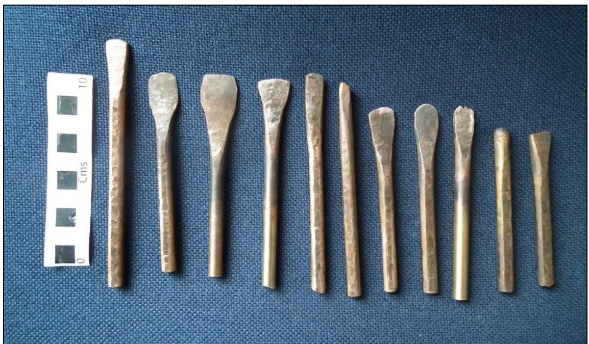
Figure 6.13 Note that the shafts of the two chisels on the left, and the chisel fifth from the left were forged with a steel hammer
