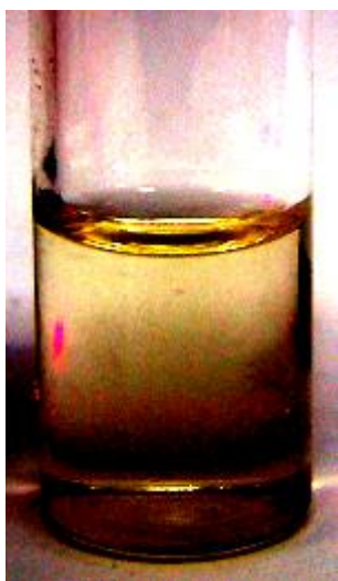
Figure A2.13: Laser scattering of ethyl valerate treated squalane sample containing 0.25% (w/w) Phenolic Antioxidant, 1% (w/w) Dispersant and 1% (w/w) Detergent
