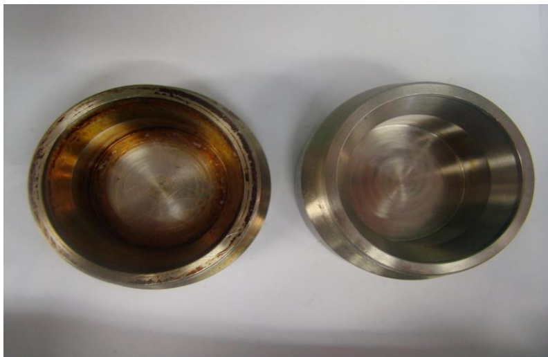
Figure 3.26: Diagram of Comparison Between a ZDDP Coated Reactor (Left Hand Side) and a Non-Coated Reactor (Right Hand Side)
