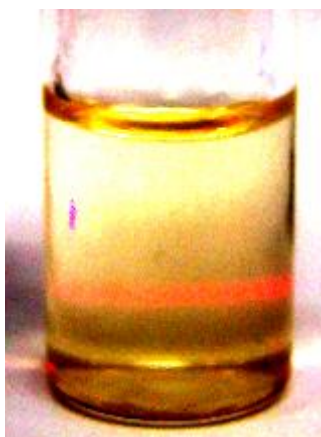
Figure A2.14: Laser scattering of 2,5-dimethylfuran treated squalane sample containing 0.25% (w/w) Phenolic Antioxidant, 1% (w/w) Dispersant and 1% (w/w) Detergent
