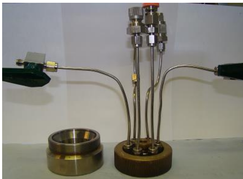
Figure 2.1: Picture of stainless steel reactor with 49 cm 3 internal volume
