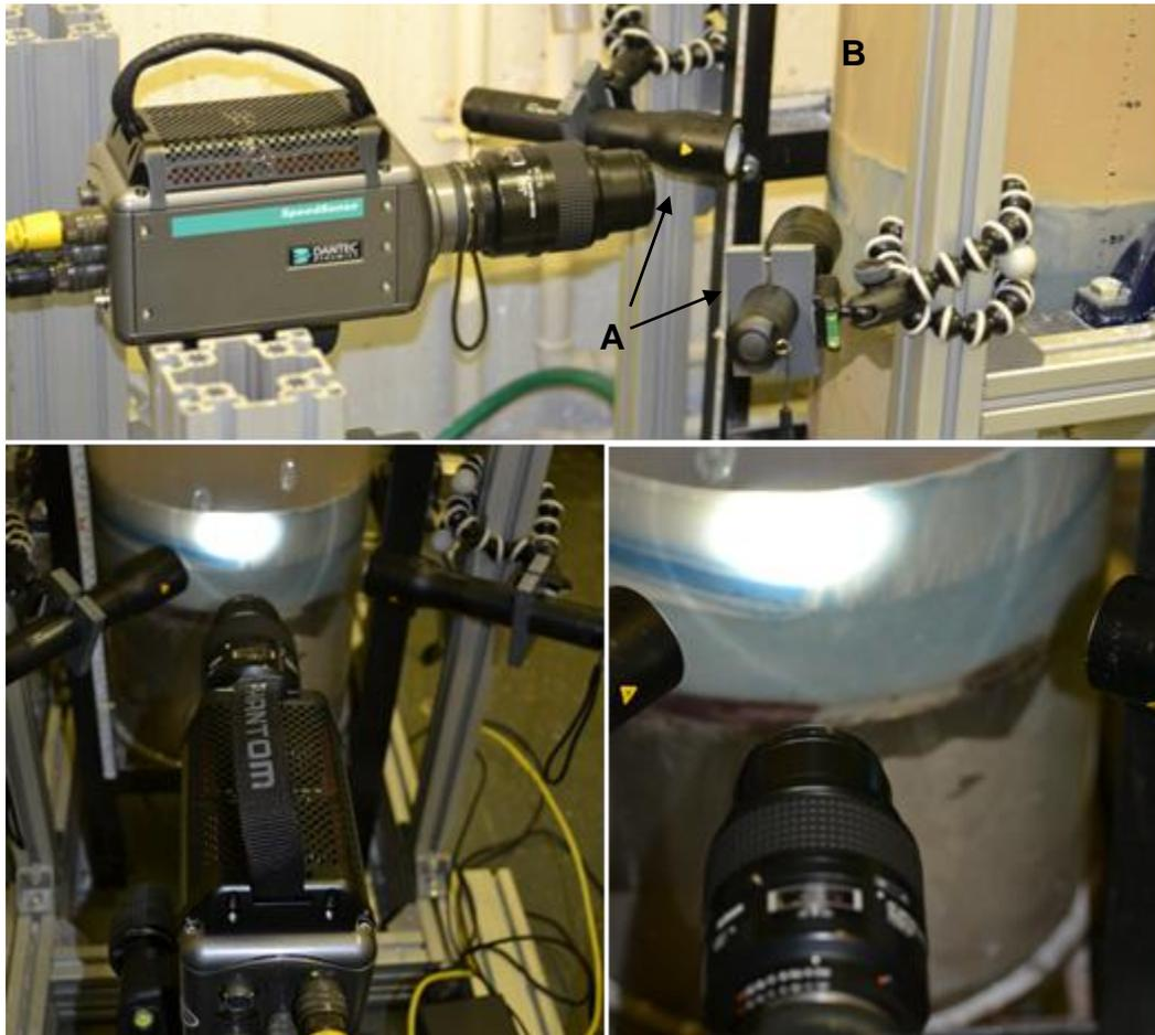
**Figure 6.8.** Photographs to demonstrate how the high speed camera and LED lights are mounted relative to the tank. **A** – Led lights, **B** – Tank wall.
