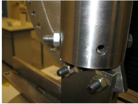
12. Position rig such that Femur head is directly under the centre of the upper loading plate.
