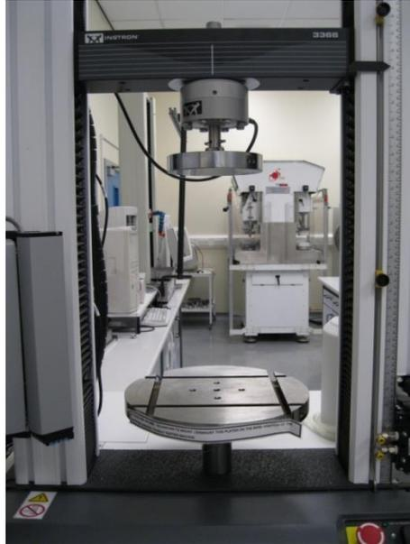
3. Turn Instron on and wait for system checks to be completed.
