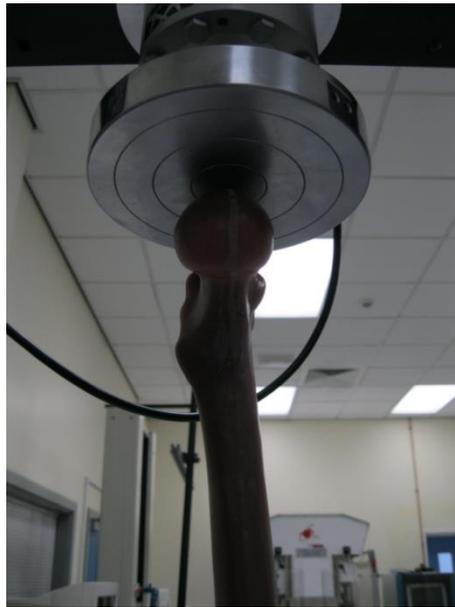
13. Secure loading rig to base plate using machining blocks with T nuts placed inside base plate grooves. N.B for best attachment, bolts should be sited as close to rig end of machining blocks as possible. The back of the machining blocks need to be at the same level or higher than at the rig end.
