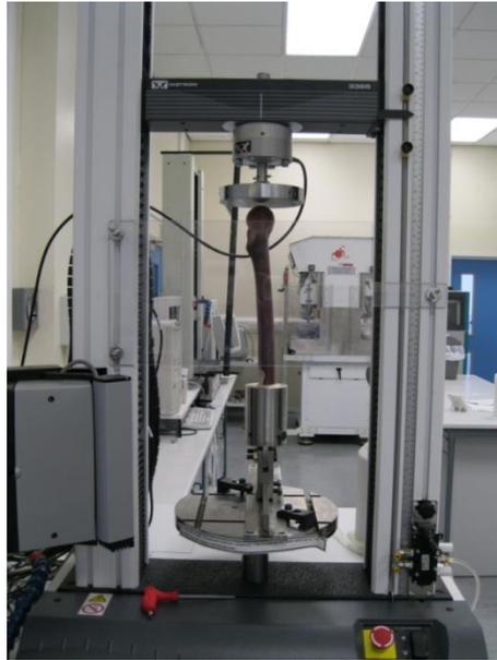
16. Move crosshead down to just above test sample
