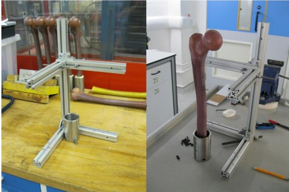
**Figure 26 The potting jig used to position the specimens within the module**
