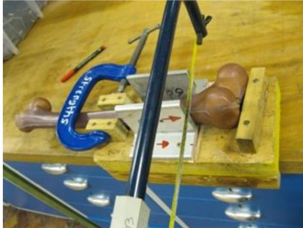
**Figure 25 Distal dissection of Sawbone Femur specimens within the cutting jig**
