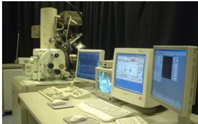
Figure 2-1 A photograph of the FIB system being used in this project, a JEOL JSM-6500F SEM combined with an Orsay Physics CANION 31 MPlus ion column.
