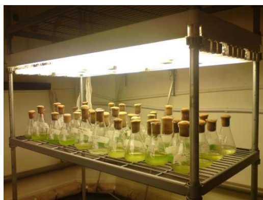
Figure 4-2 Illuminated algal cultures in temperature-controlled growth room
