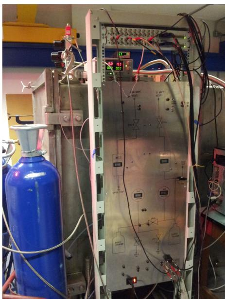
Figure 7.2: Photograph of the DRIFT-IIe gas mixing system front panel.
