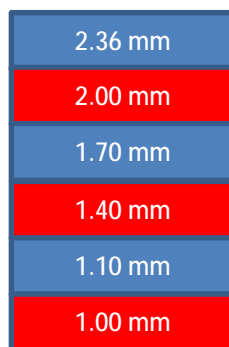
Fig. 2.1, The order of the sieves used to separate the particles size.
