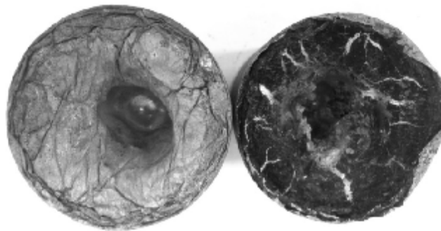
Fig. 2.8, Top part of the molten aluminium- Left melted under argon gas- Right- melted under atmospheric air
