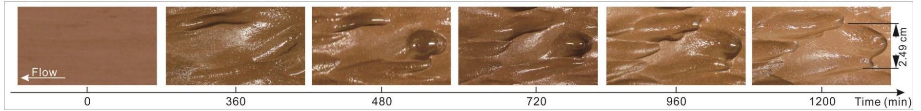
Figure 6.21 Evolution of flute with internal secondary structure. It was observed in the clay bed of Exp. 7. Flow from right to left.
