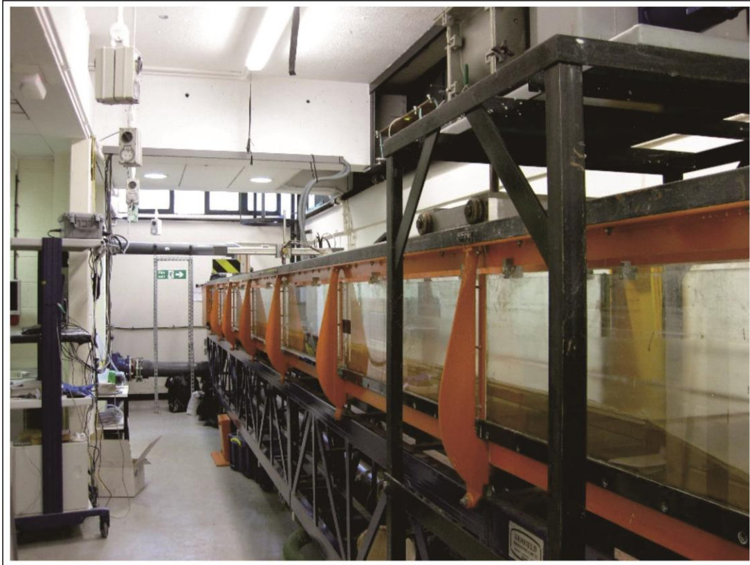
Figure 3.1 The recirculating Hydraulic Slurry Flume in the Sorby Environment Fluid Dynamics Laboratory; looking downstream. The false floor composed of Perspex can be clearly seen.
