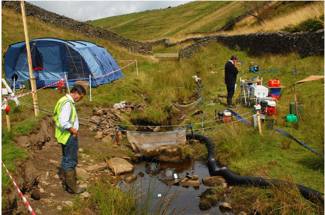
Figure 6.1 Stream section being prepared for electric shock treatment
