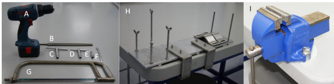
Figure 2.1 Dissection equipment. A – Hand held power drill. B – Metal File. C – Smooth corer. D – Serrated corer. E – Serrated corer drill attachment. F – Scalpel. G – Hack saw. H – Clamping apparatus to hold large limbs in place. I – Bench top vice for holding smaller limbs in place.
