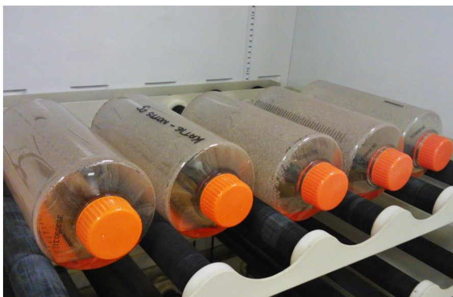
Figure 2-1. Roller bottles in roller bottle incubator
