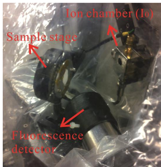
Figure 4.10 Photograph of the sample environment filled with helium gas. The propagation path of the X-ray was fully covered by helium gas, to reduce the scattering and absorption of soft fluorescent X-ray by air.
