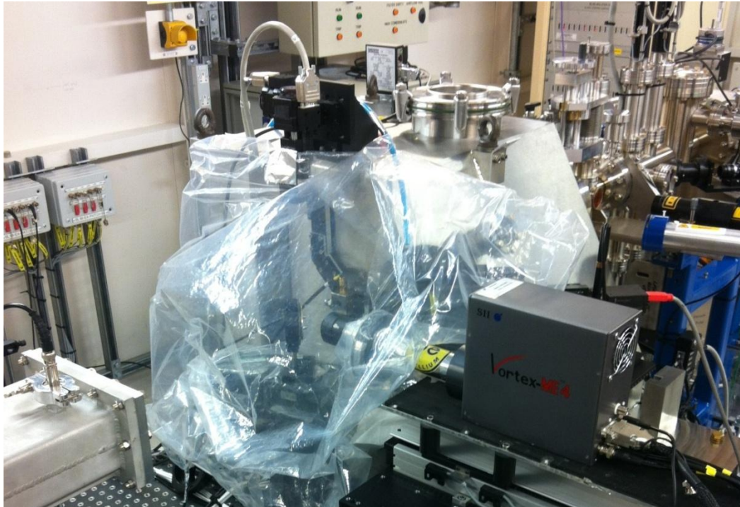
Figure 4.9 The instrumental set-up at beamline I18 of Diamond Light Source. The incident X-ray beam produced from the storage ring comes from the upper right side in the photo.
