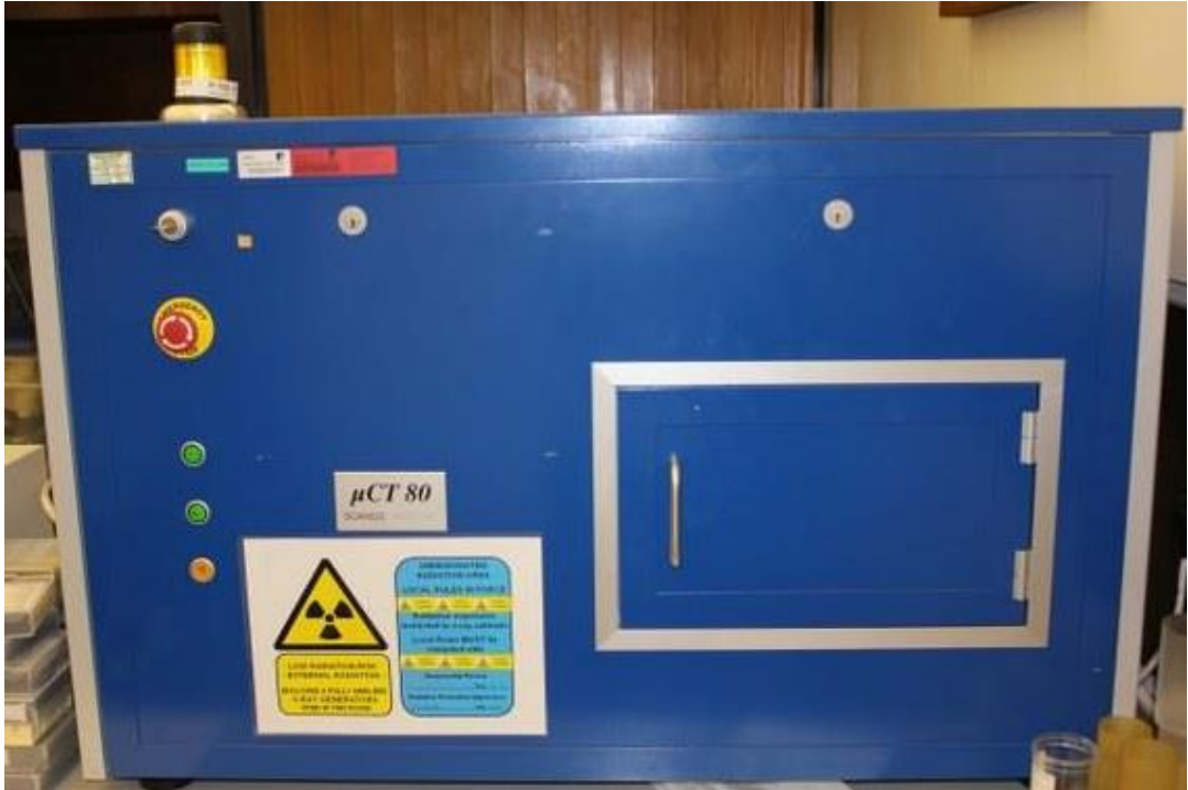
Figure 4.8. \mu -CT 80 Scanco Machine.
