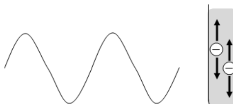
Figure 2.8: Ionic conduction – charged particles in reaction mixture will follow the applied electric field adapted from reference [49]
