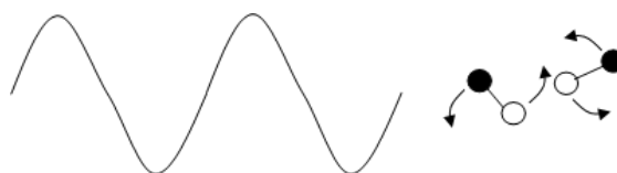
Figure 2.7: Dipolar interaction – dipolar molecules in reaction mixture will try to align with an oscillating electric field adapted from reference [49]
