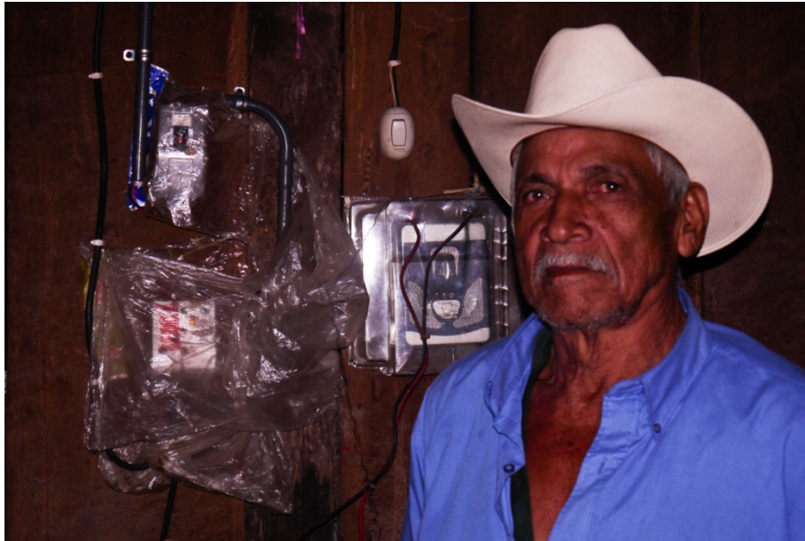
Figure 5-19: Leoncio Gonzalez, an end-user of a 55W PV household system with his well-protected electronic components.
