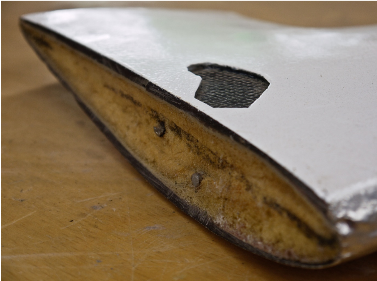
Figure 4-27: WindAid's new foam core glass-fibre blades with two steel spars and an outer layer of carbon fibre.
