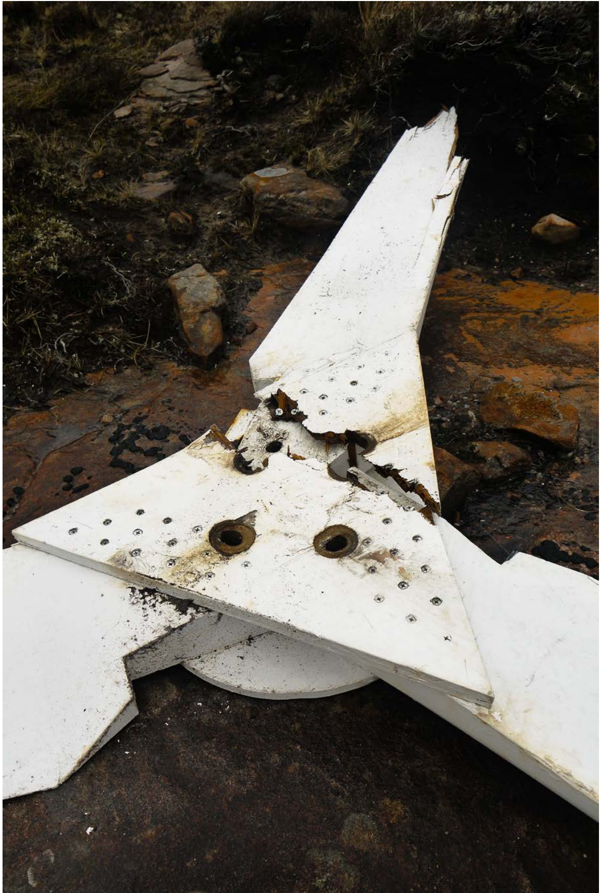
Figure 6-1: A shattered set of wind turbine blades lies abandoned amongst the heather and rocks that cover the majority of this windswept peninsula
