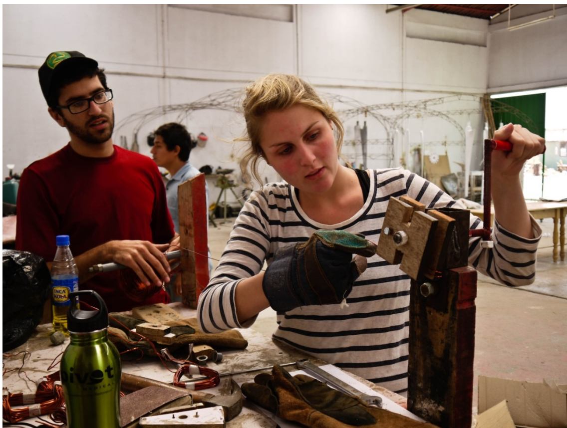
Figure 4-11: A British volunteer winds coils for the generator under the supervision of Cuban-American and Peruvian permanent staff members.
