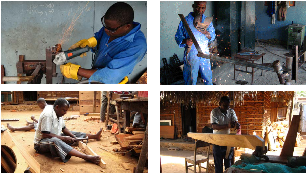
Figure 2-5: Manufacture of a SWT using simple tools and techniques in Mozambique. Photo courtesy of The Clean Energy Initiative.
