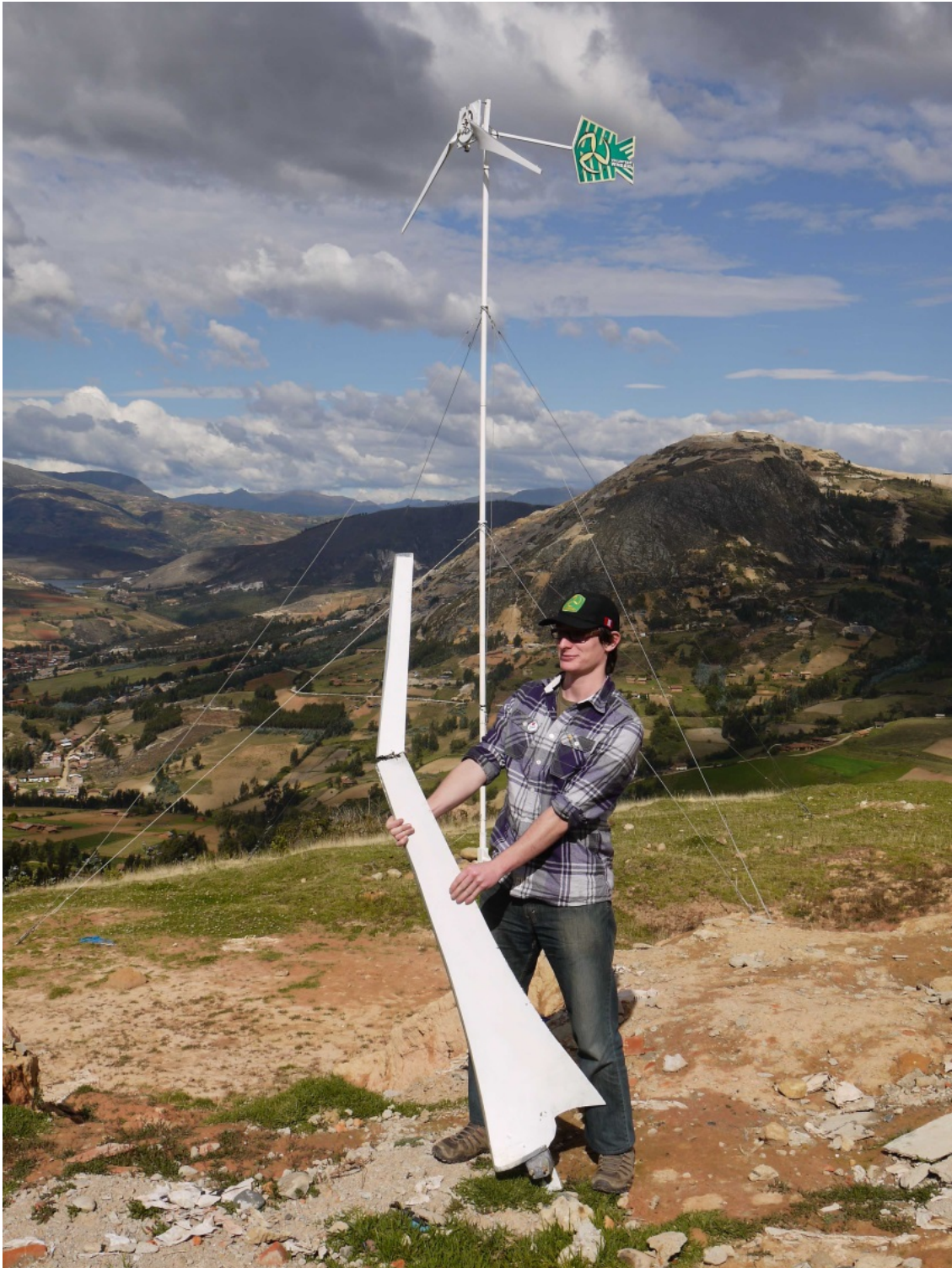
Figure 4-1: The author holding a broken blade that flew off of the 2.5kW wind turbine installed in the Andean community of Paranchique by WindAid.
