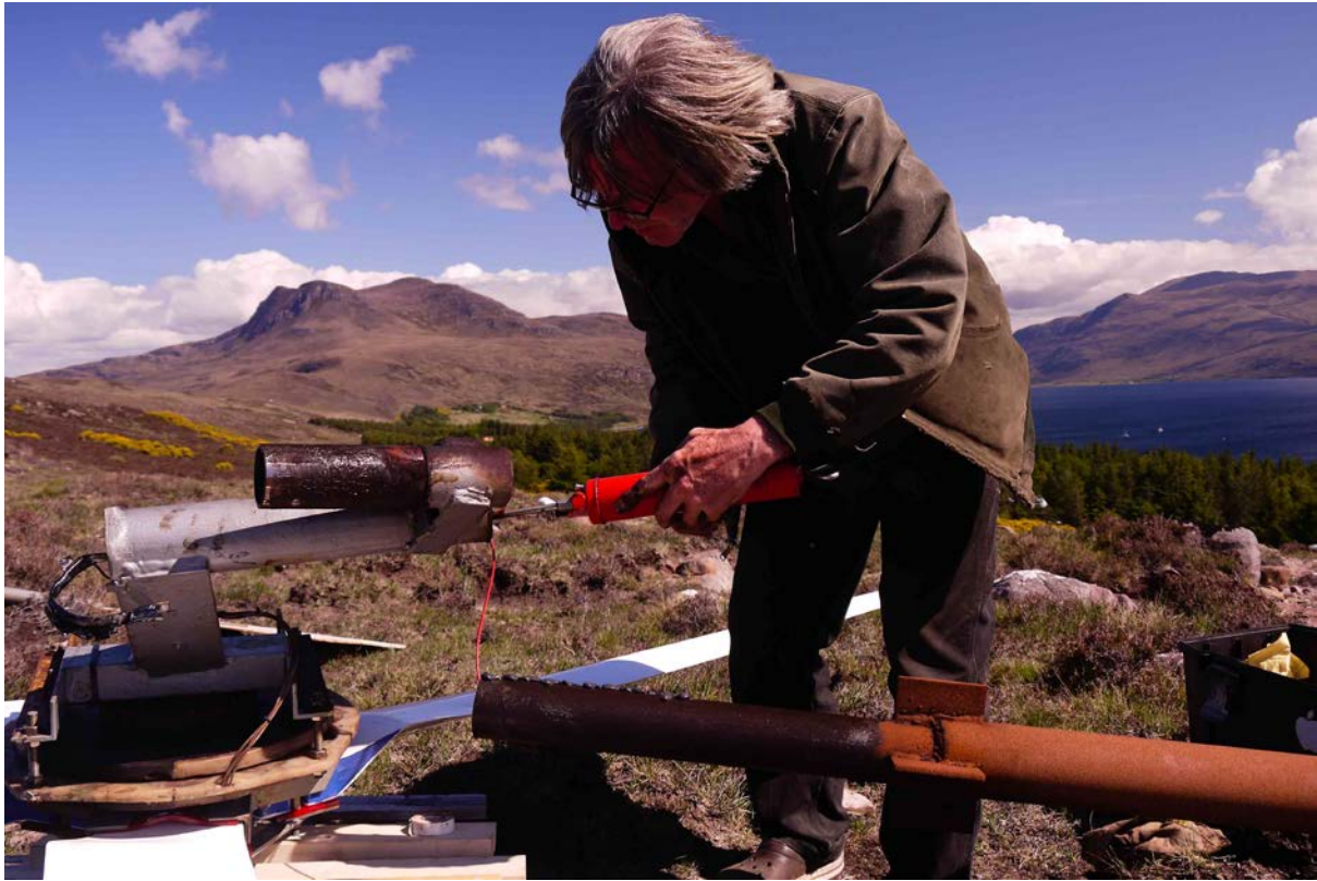
Figure A-9: Re-greasing the yaw bearing to enable it to follow the wind more easily.
