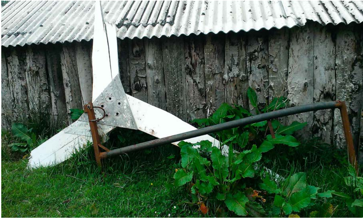
Figure 6-32: What's left of the blades after colliding with the tail in 2011.
