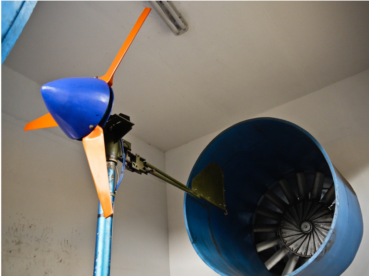
Figure 4-26: An IT-PE-100 in the wind tunnel been constructed by Soluciones Prácticas at the Universidad Nacional de Ingeniería in Lima.
