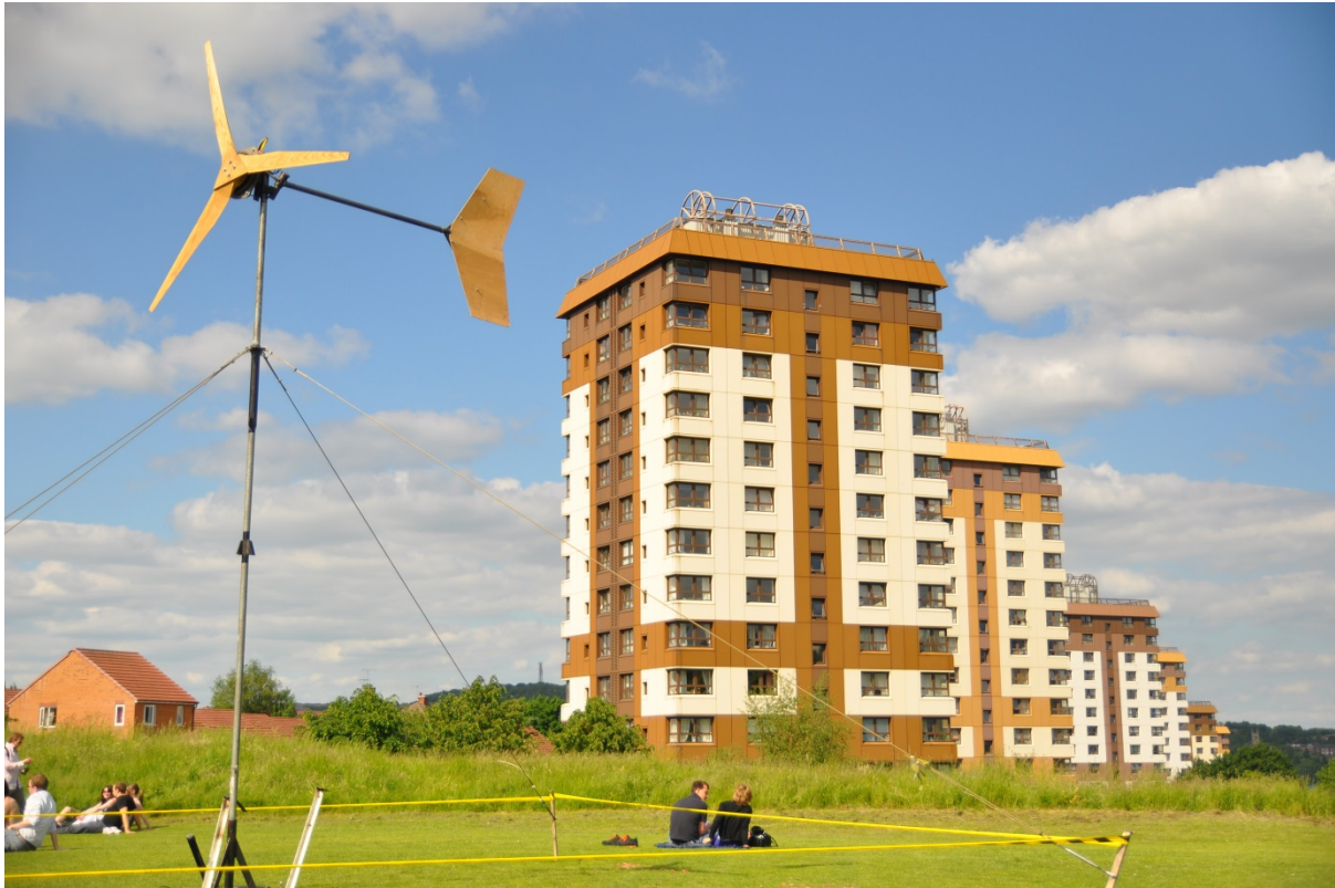
Figure 3-10: The EWB-Sheffield 2.4m Piggott turbine on display at the Peace in the Park festival in Sheffield in 2010. Photo courtesy of Pete Hodge.
