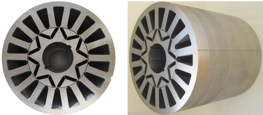
(a) Stacks of stator and rotor laminations
