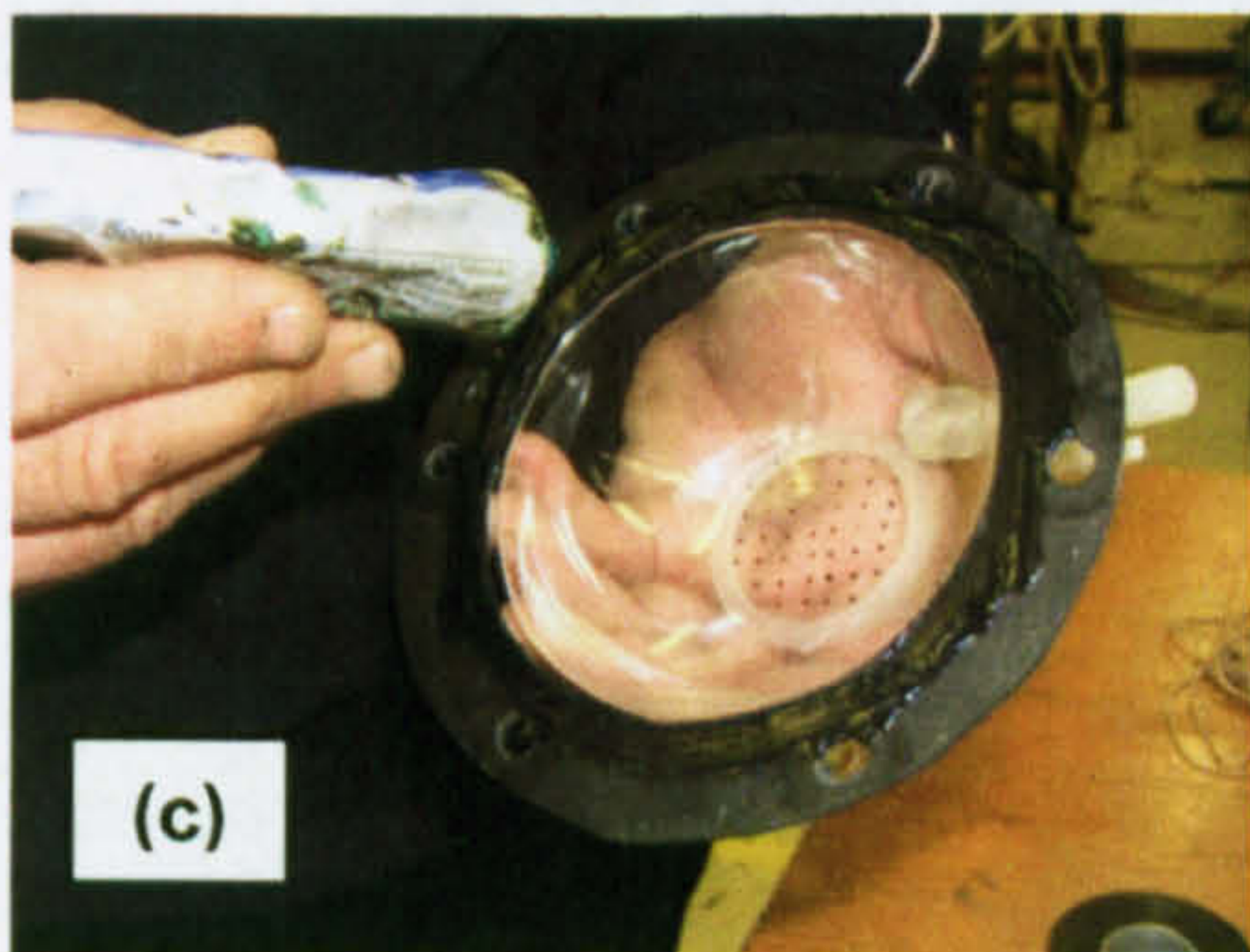
Figure 4.27. The procedure of model assembly. (a) lay the latex covering the top of the dome; (b) compress the latex by compression ring and plot the ink on the membrane for grid, the luer was screw into the base covered by PVC insulation tape; (c) attach the rubber ring on the dome and glue (Hylomar Universal Blue) to stick the contact surfaces; (d) fix the valve on the luer to set up a drainage system, and use epidemic syringe to inject the water into the globe.
