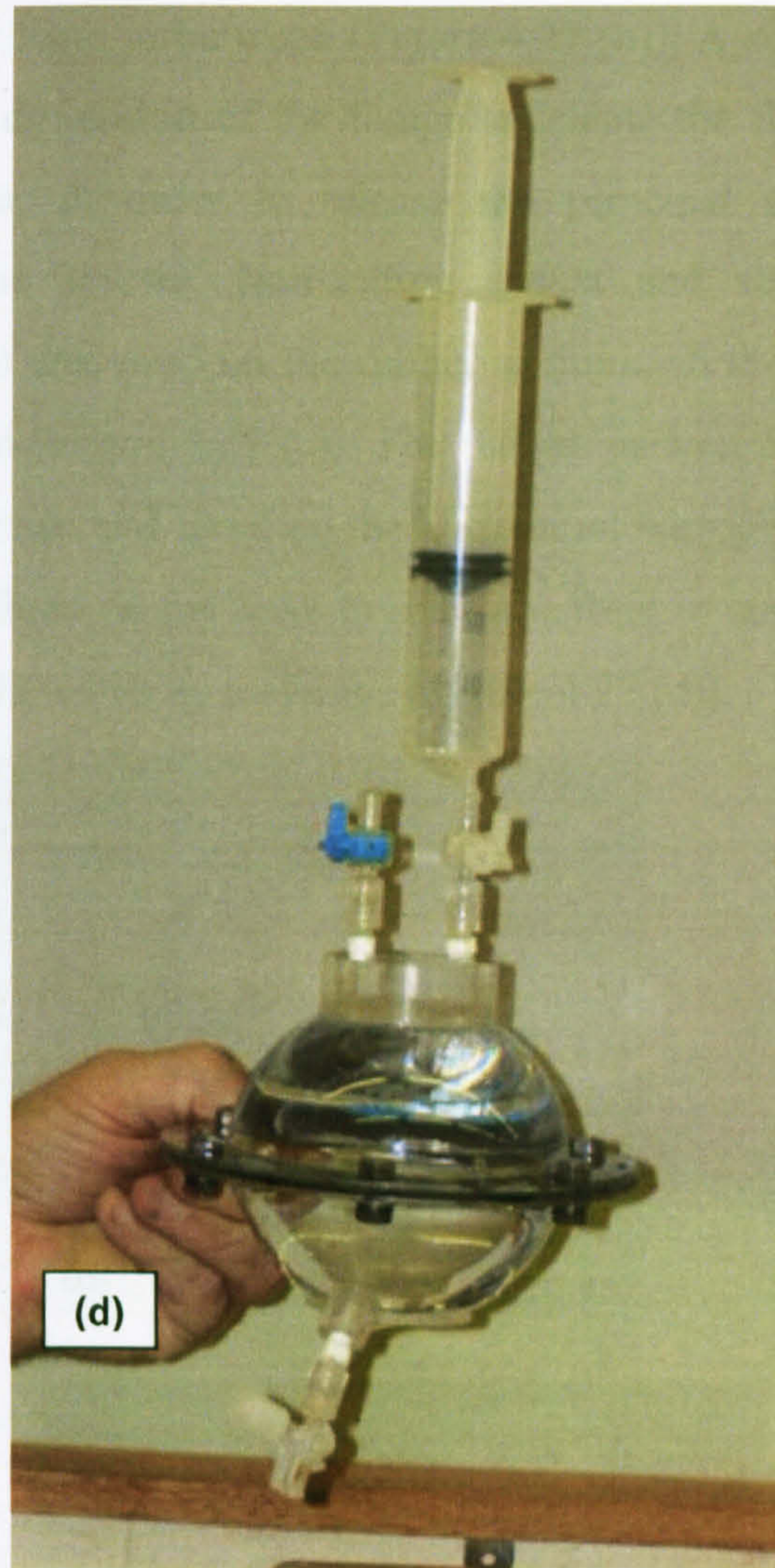
Figure 4.27. The procedure of model assembly. (a) lay the latex covering the top of the dome; (b) compress the latex by compression ring and plot the ink on the membrane for grid, the luer was screw into the base covered by PVC insulation tape; (c) attach the rubber ring on the dome and glue (Hylomar Universal Blue) to stick the contact surfaces; (d) fix the valve on the luer to set up a drainage system, and use epidemic syringe to inject the water into the globe.
