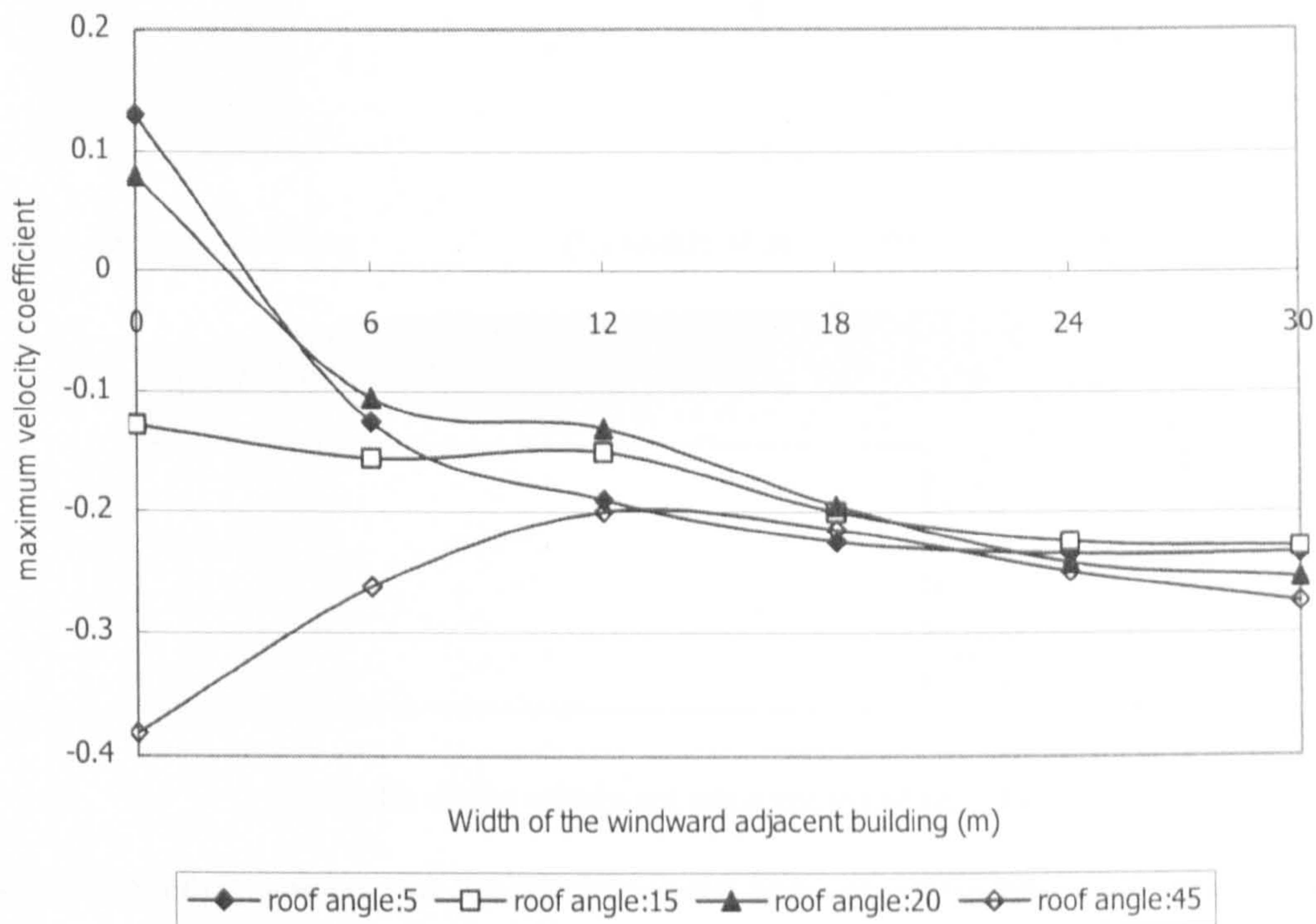
Figure 5.38: Relationship between the maximum air velocity coefficient and the width of the windward adjacent building
