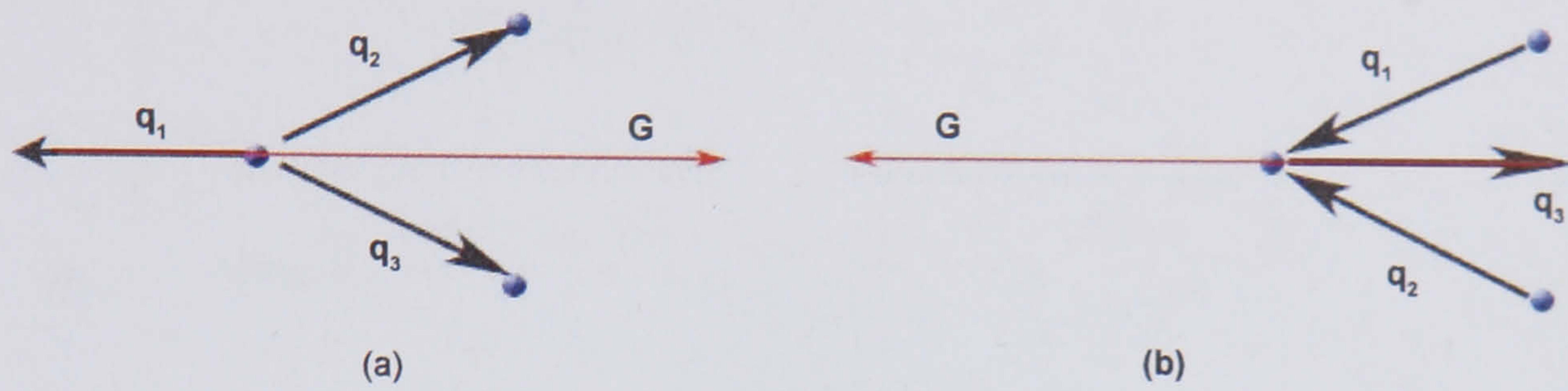
Figure 2.10: Umklapp scattering vector diagram of (a) decay process and (b) merge process.
