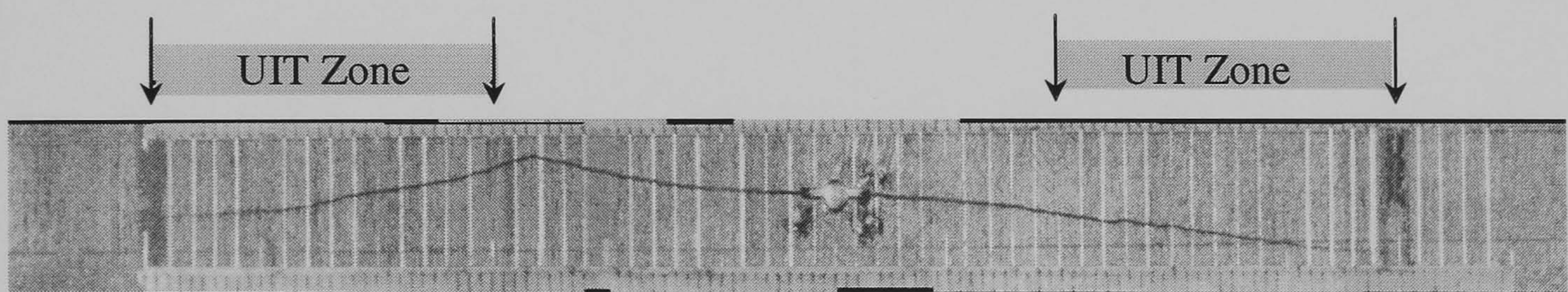
Figure 5.44 Crack growth pattern in a M(T) specimen made of Al 2024-T3 pointed out the position of treated zone in every side of the notch tip. Last photo obtained before the specimen fractured.
